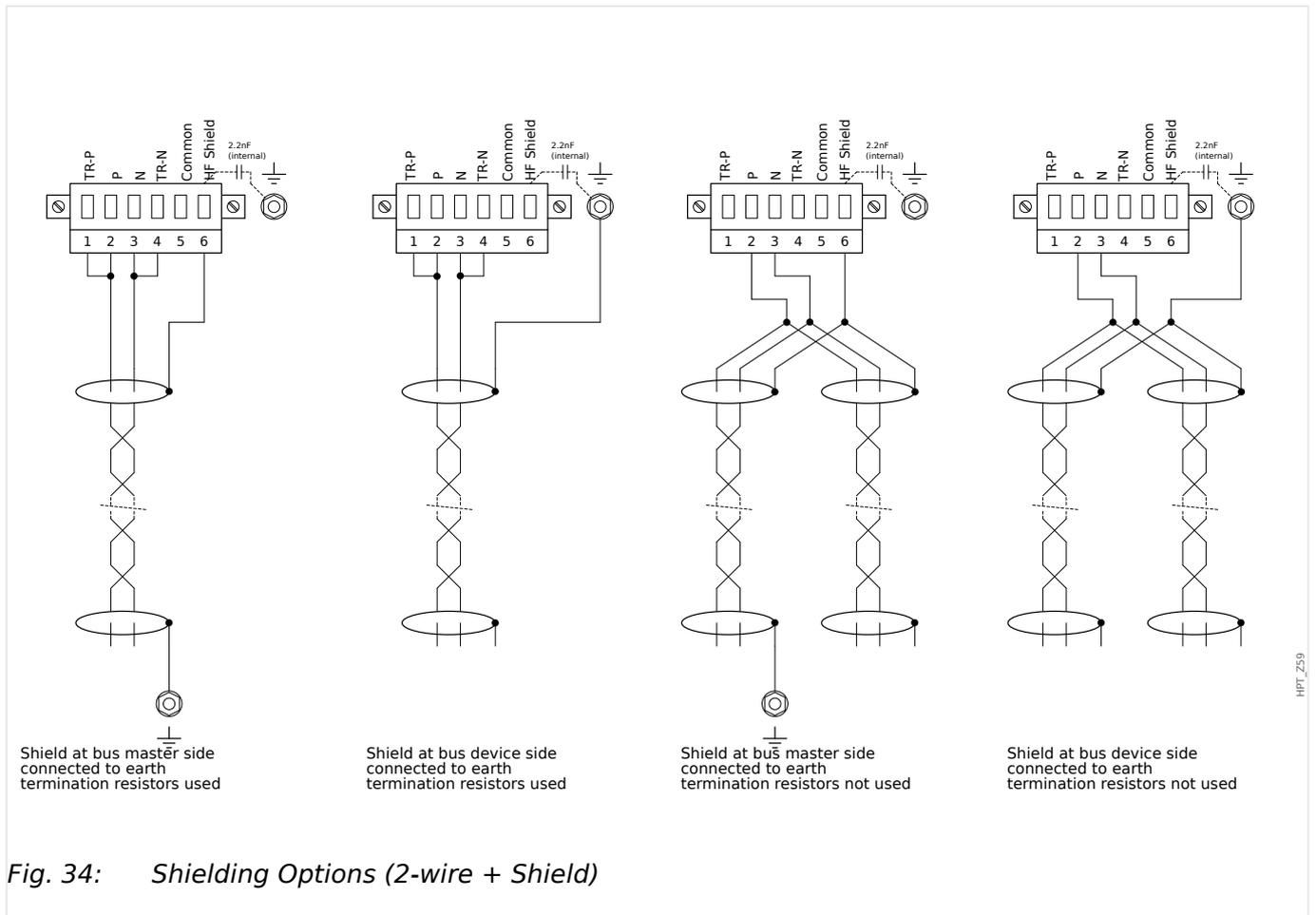
Fig. 34: Shielding Options (2-wire + Shield)
