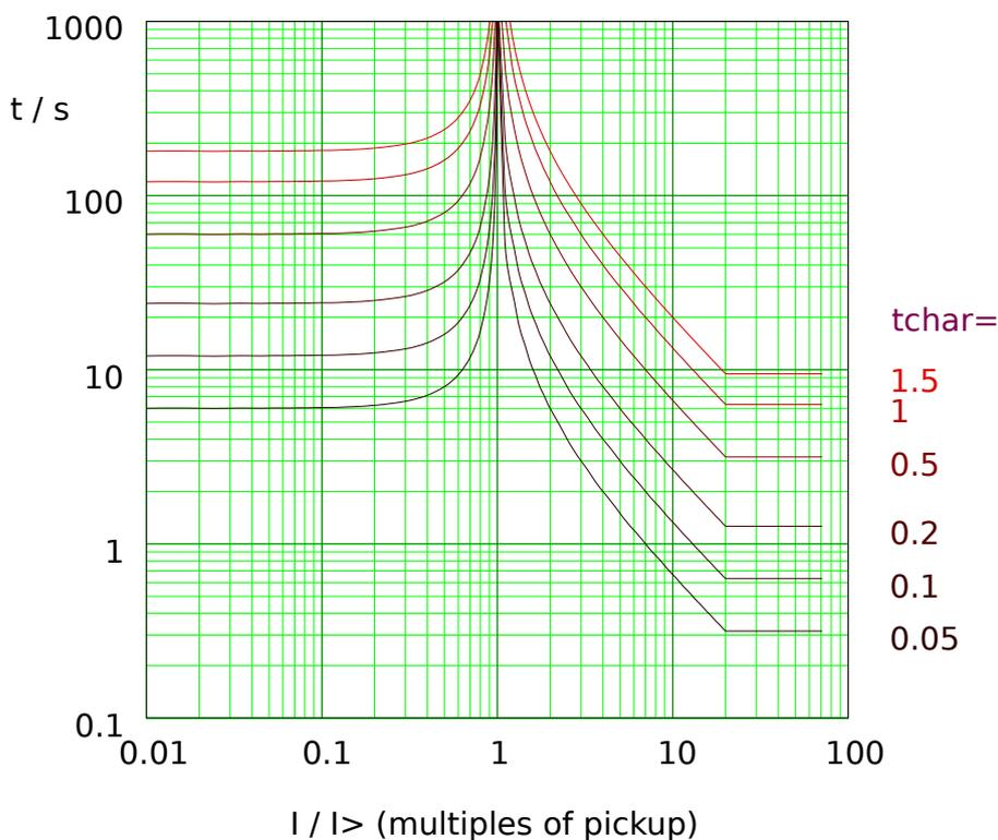
Fig. 48: LINV: reset delay (left half,  $I < I>$ ) and trip delay (right half,  $I > I>$ ), example for  $I_{max} = 20 \cdot I>$ .
