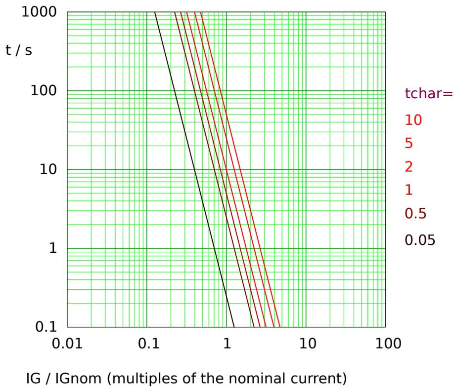
Fig. 69: I4T tripping curve, example diagram for measured (non-sensitive) earth/ground current (51G). Note that only the range  $I_G > I_G>$  is actually effective.
