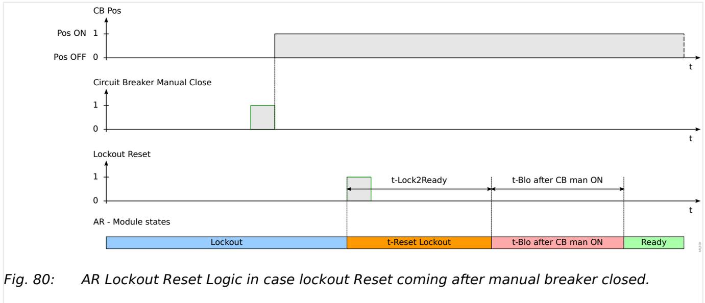
Fig. 80: AR Lockout Reset Logic in case lockout Reset coming after manual breaker closed.
