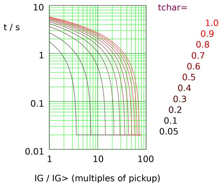
Fig. 65: RXIDG: trip delay,  $I_G > I_{G>}$ .
