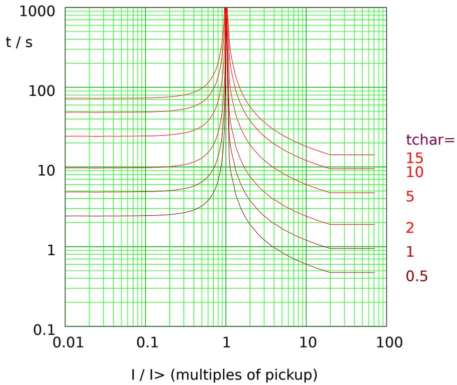
Fig. 49: MINV: reset delay (left half,  $I < I>$ ) and trip delay (right half,  $I > I>$ ), example for  $I_{max} = 20 \cdot I>$ .
