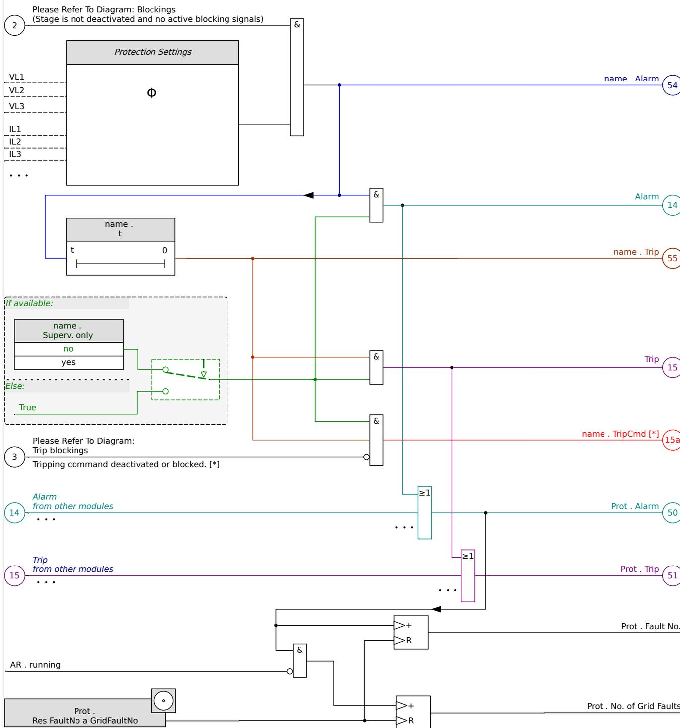
Fig. 43: Rough sketch of the functionality of any HighPROTEC protective element.
