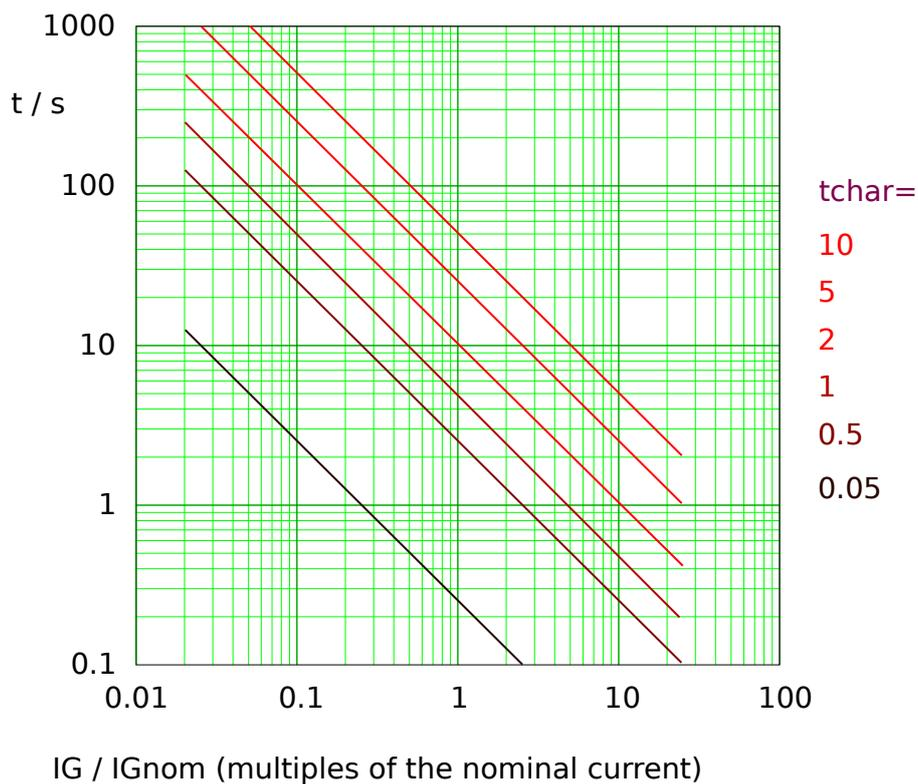
Fig. 67: IT tripping curve, example diagram for measured (non-sensitive) earth/ground current ( $5I_G$ ). Note that only the range  $I_G > I_G>$  is actually effective.
