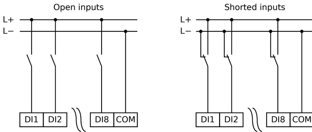
Fig. 105: Safe State of the Digital Inputs
