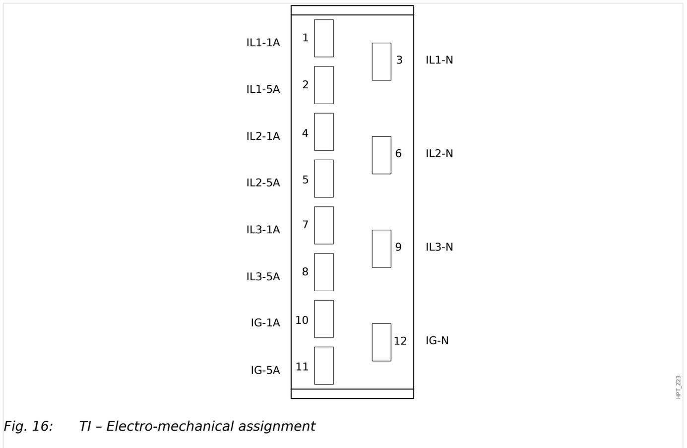
Fig. 16: TI - Electro-mechanical assignment
