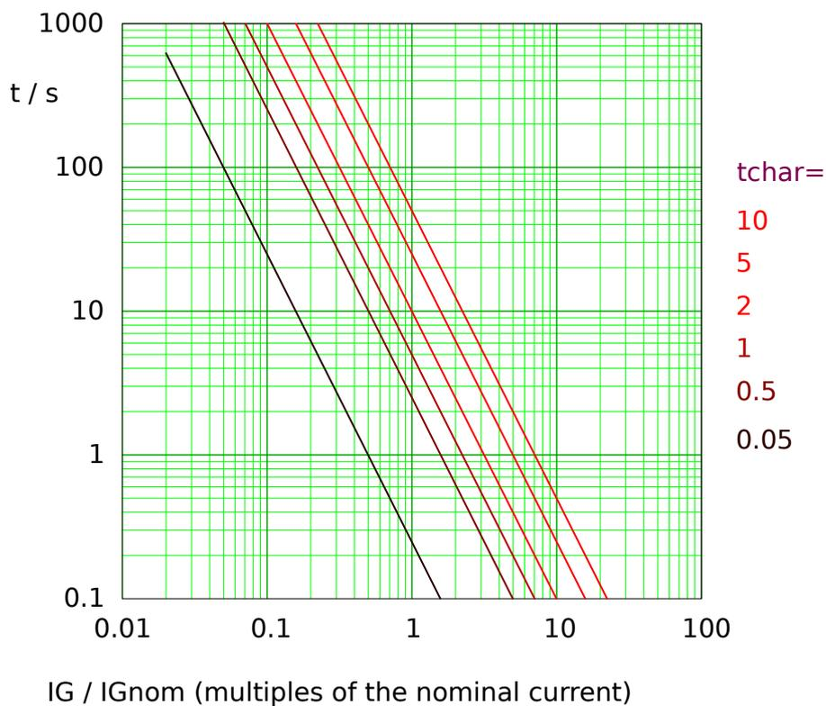
Fig. 68: I2T tripping curve, example diagram for measured (non-sensitive) earth/ground current ( $5I_G$ ). Note that only the range  $I_G > I_G>$  is actually effective.
