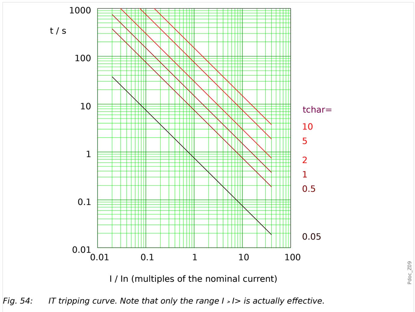
Fig. 54: IT tripping curve. Note that only the range  $I > I_n$  is actually effective.
