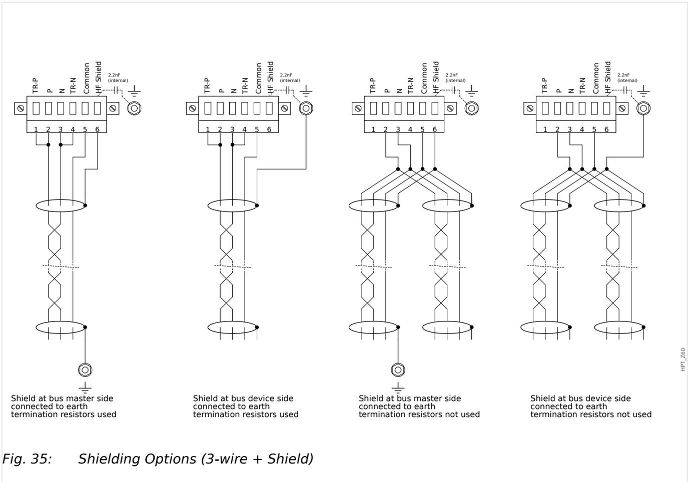
Fig. 35: Shielding Options (3-wire + Shield)
