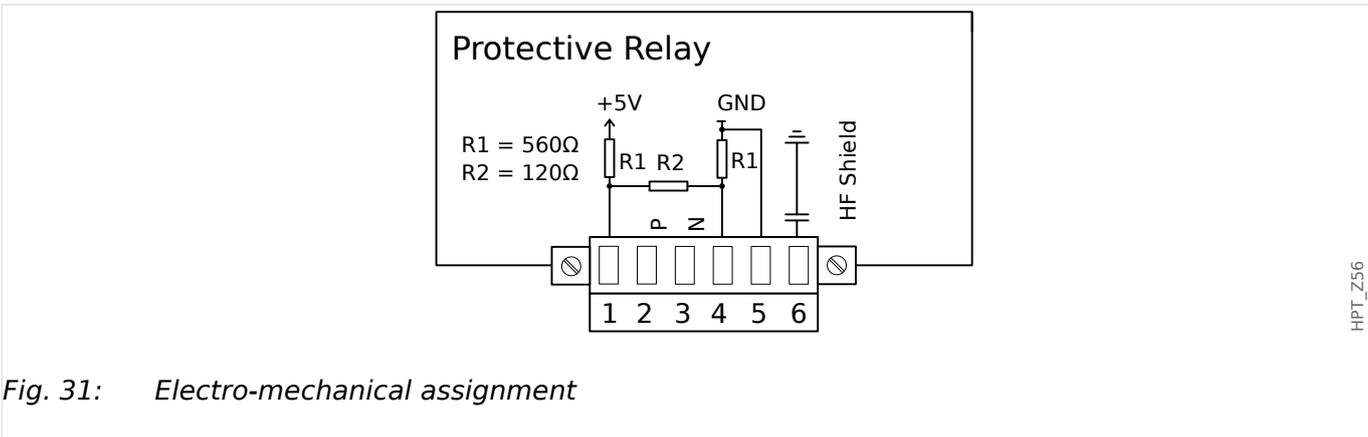
Fig. 31: Electro-mechanical assignment
