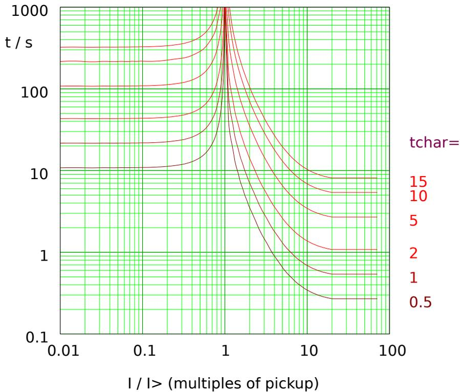
Fig. 50: VINV: reset delay (left half,  $I < I>$ ) and trip delay (right half,  $I > I>$ ), example for  $I_{max} = 20 \cdot I>$ .
