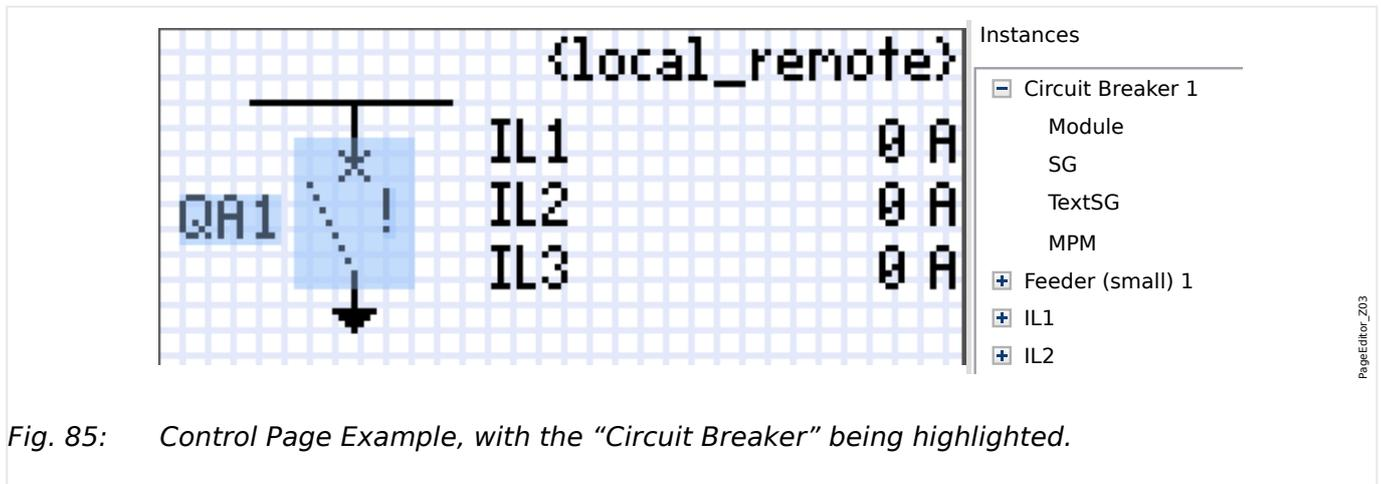
Fig. 85: Control Page Example, with the “Circuit Breaker” being highlighted.
