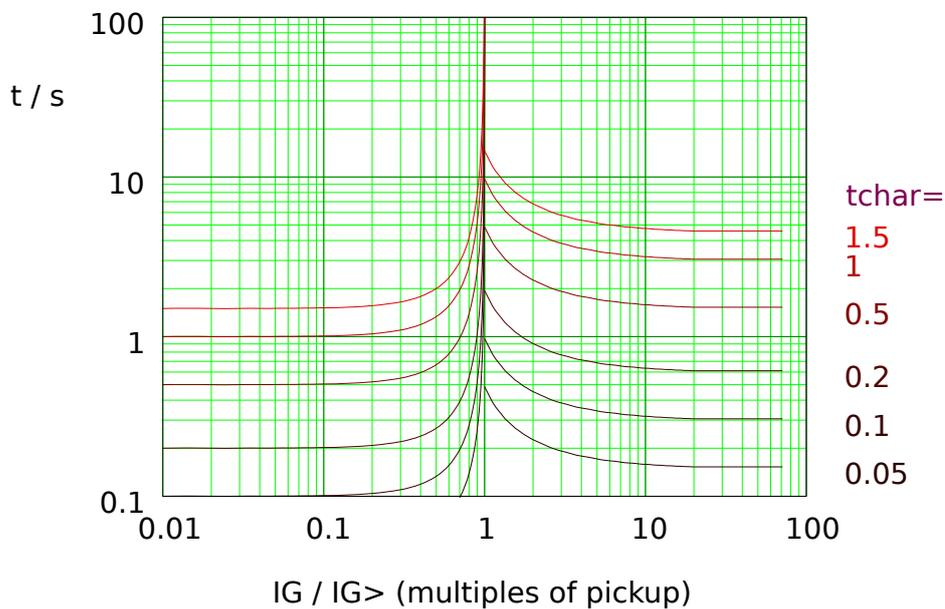
Fig. 64: RINV: reset delay (left half,  $I_G < I_{G>}$ ) and trip delay (right half,  $I_G > I_{G>}$ ), example for  $I_{G,max} = 20 \cdot I_{G>}$ .
