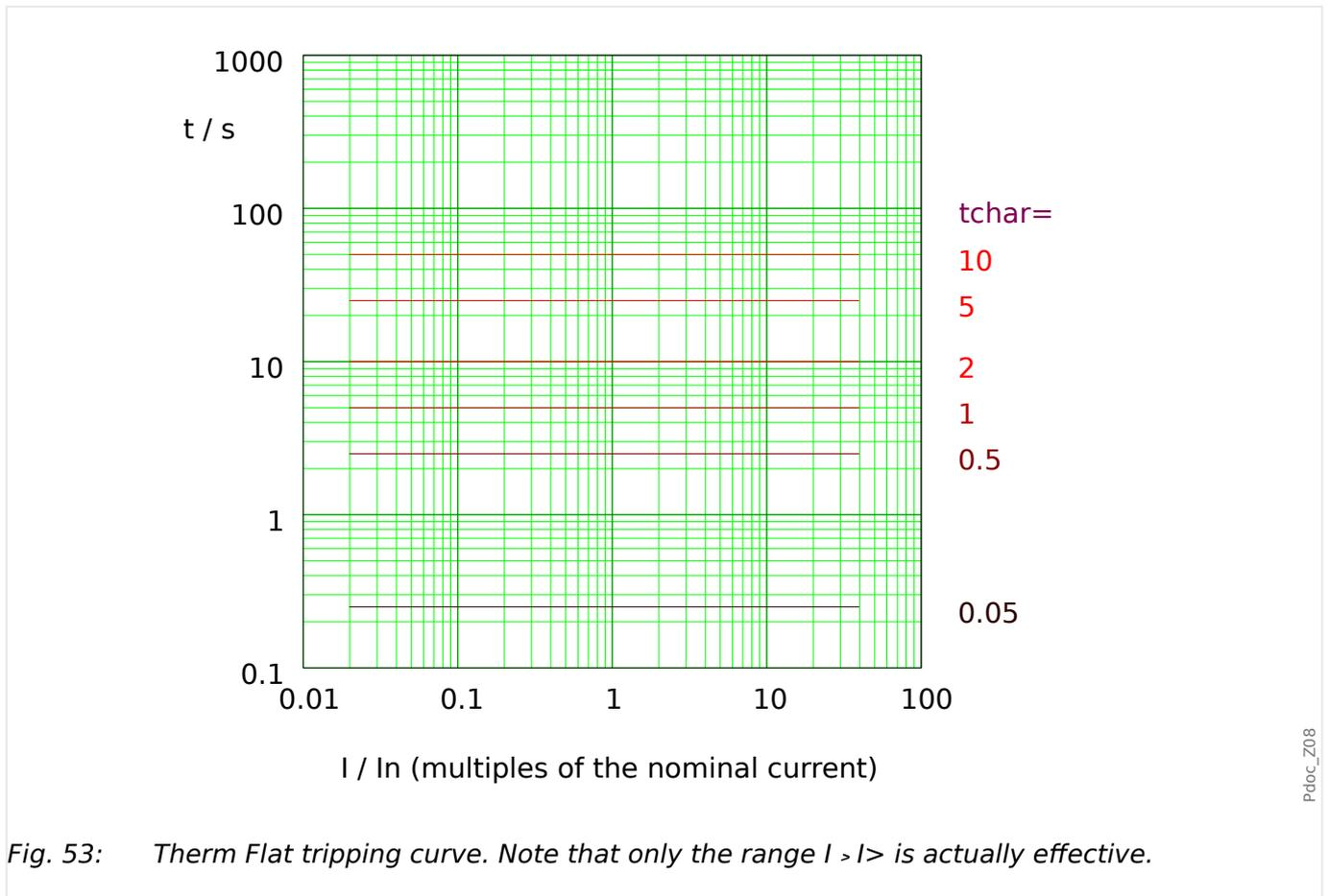
Fig. 53: Therm Flat tripping curve. Note that only the range  $I > I_n$  is actually effective.
