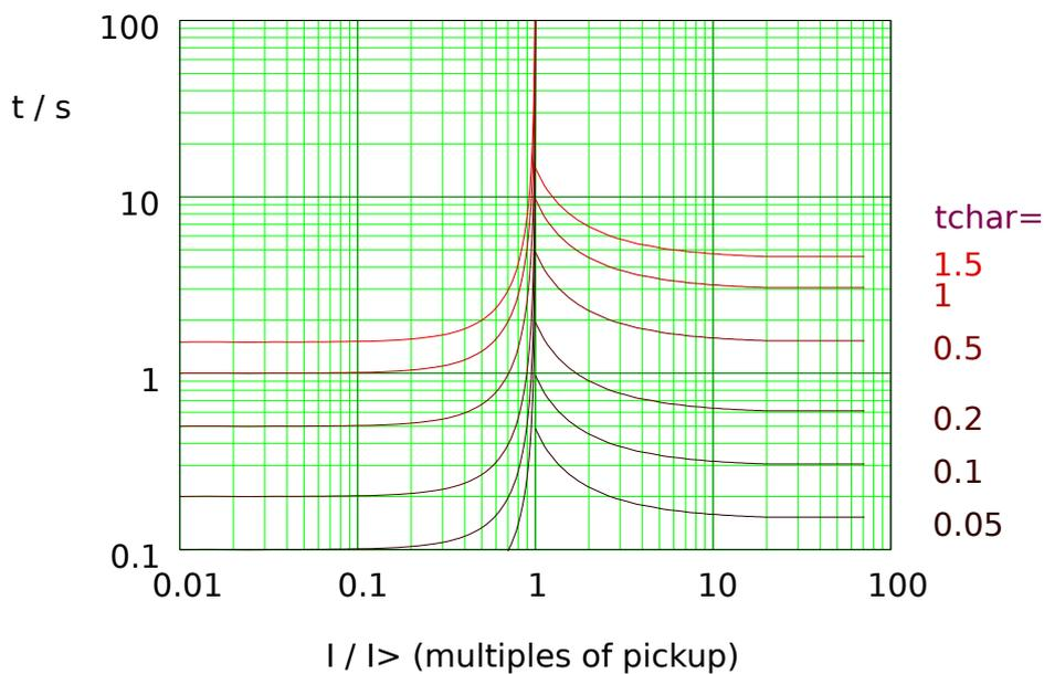
Fig. 52: RINV: reset delay (left half,  $I < I>$ ) and trip delay (right half,  $I > I>$ ), example for  $I_{max} = 20 \cdot I>$ .
