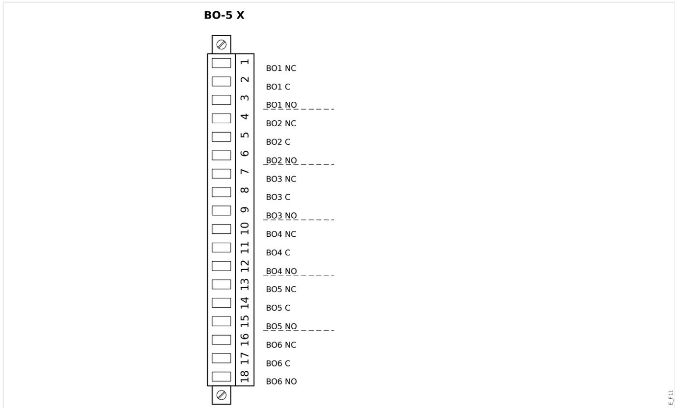
Fig. 13: RO-5 - Pin Assignment
