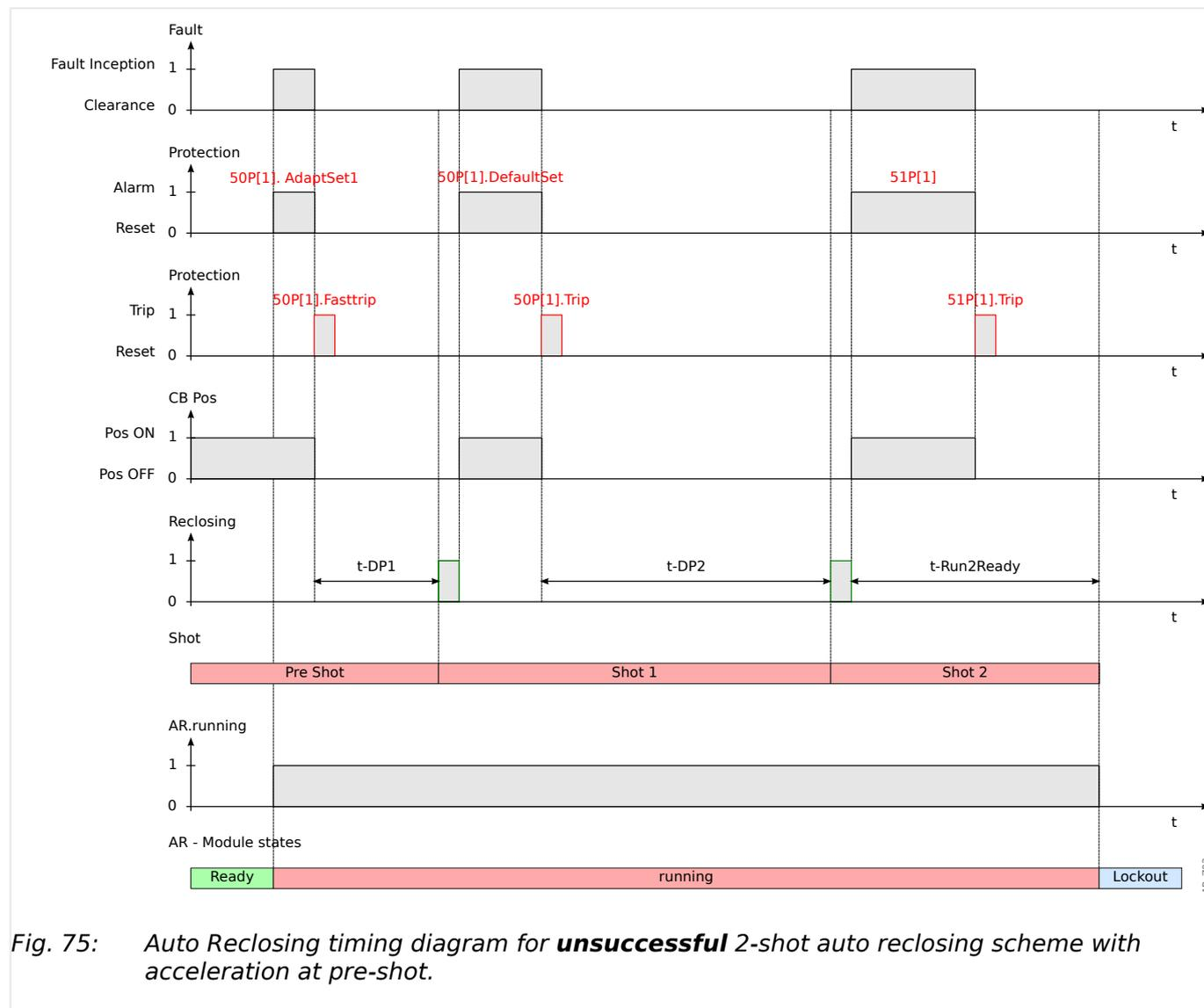
Fig. 75: Auto Reclosing timing diagram for **unsuccessful** 2-shot auto reclosing scheme with acceleration at pre-shot.
