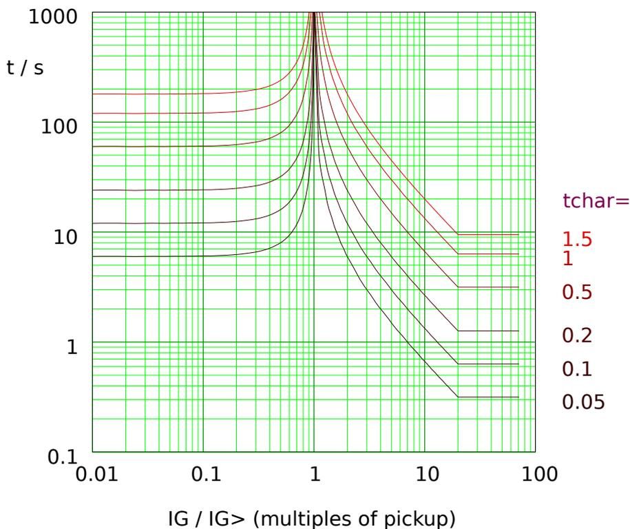
Fig. 60: LINV: reset delay (left half,  $I_G < I_{G>}$ ) and trip delay (right half,  $I_G > I_{G>}$ ), example for  $I_{G,max} = 20 \cdot I_{G>}$ .
