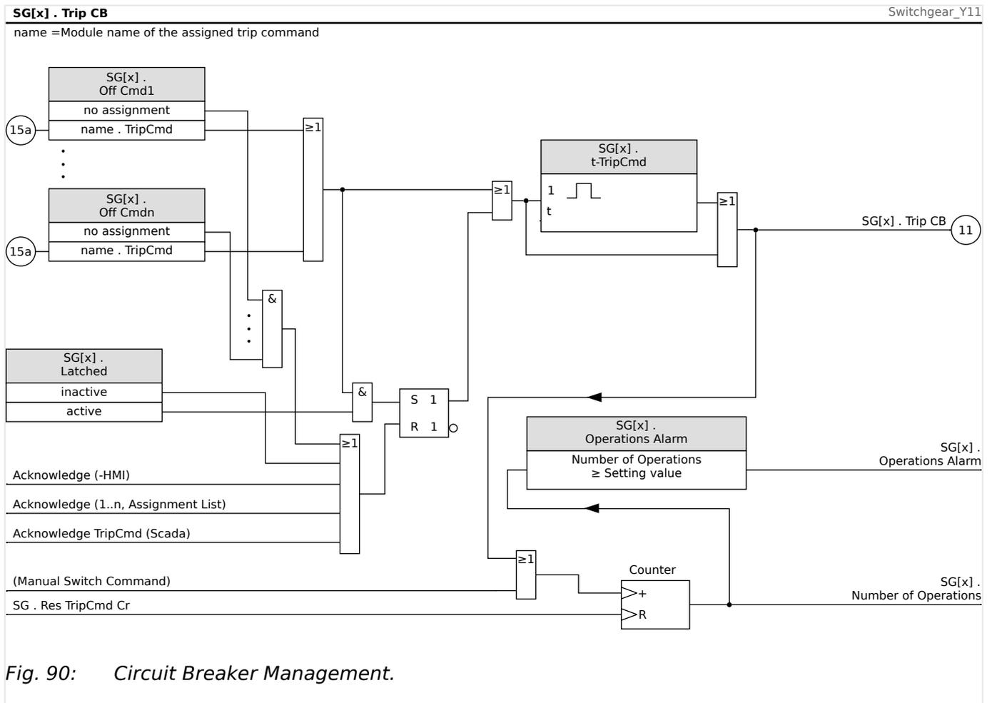
Note that in the diagram above, “SG[x]” represents “switchgear number x”; however, the exact designation is defined in the single-line file, see also [↪](#) “Single-Line Diagram”.
