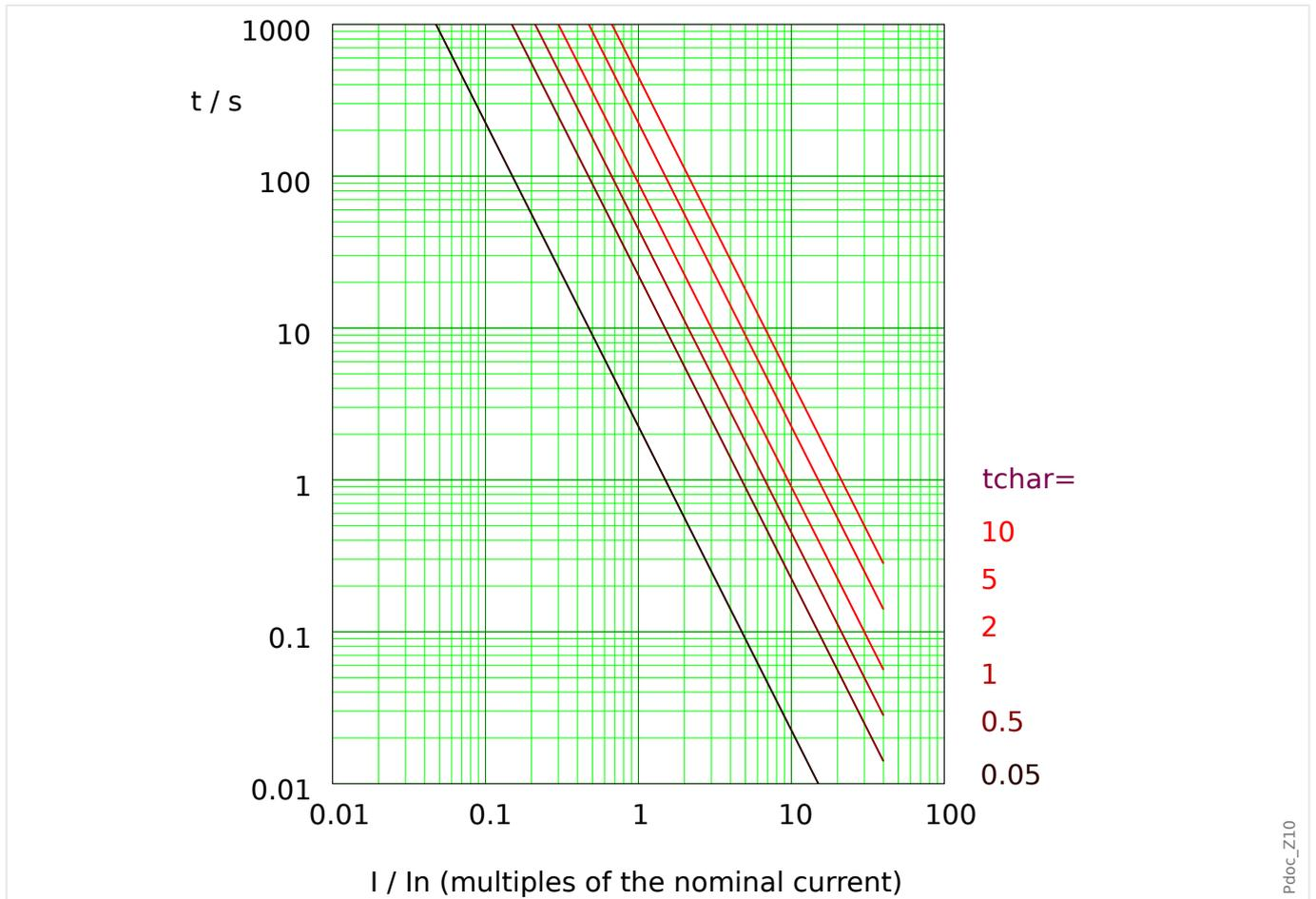
Fig. 55: I2T tripping curve. Note that only the range  $I > I_n$  is actually effective.
