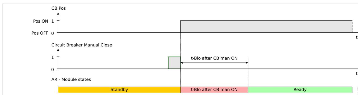
Fig. 77: Auto Reclosing States during manual breaker closing.
