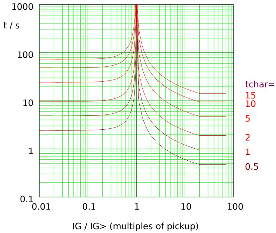
Fig. 61: MINV: reset delay (left half,  $I_G < I_{G>}$ ) and trip delay (right half,  $I_G > I_{G>}$ ), example for  $I_{G,max} = 20 \cdot I_{G>}$ .
