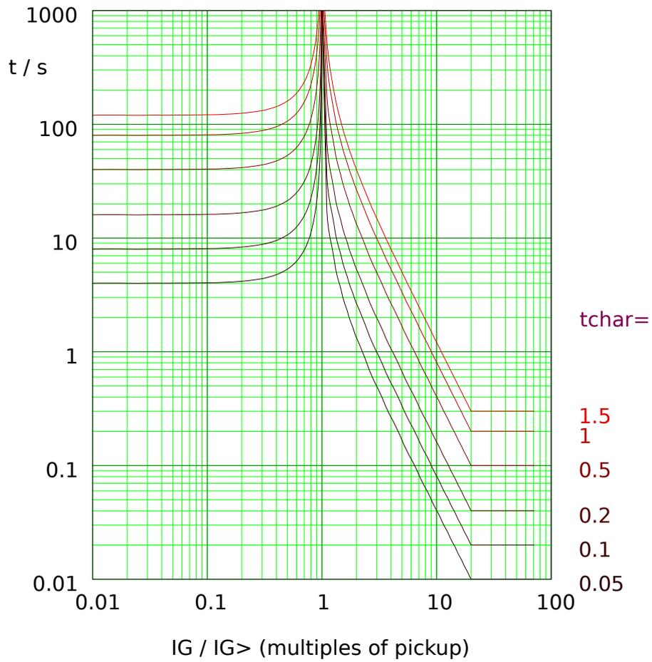
Fig. 59: EINV: reset delay (left half,  $I_G < I_{G>}$ ) and trip delay (right half,  $I_G > I_{G>}$ ), example for  $I_{G,max} = 20 \cdot I_{G>}$ .
