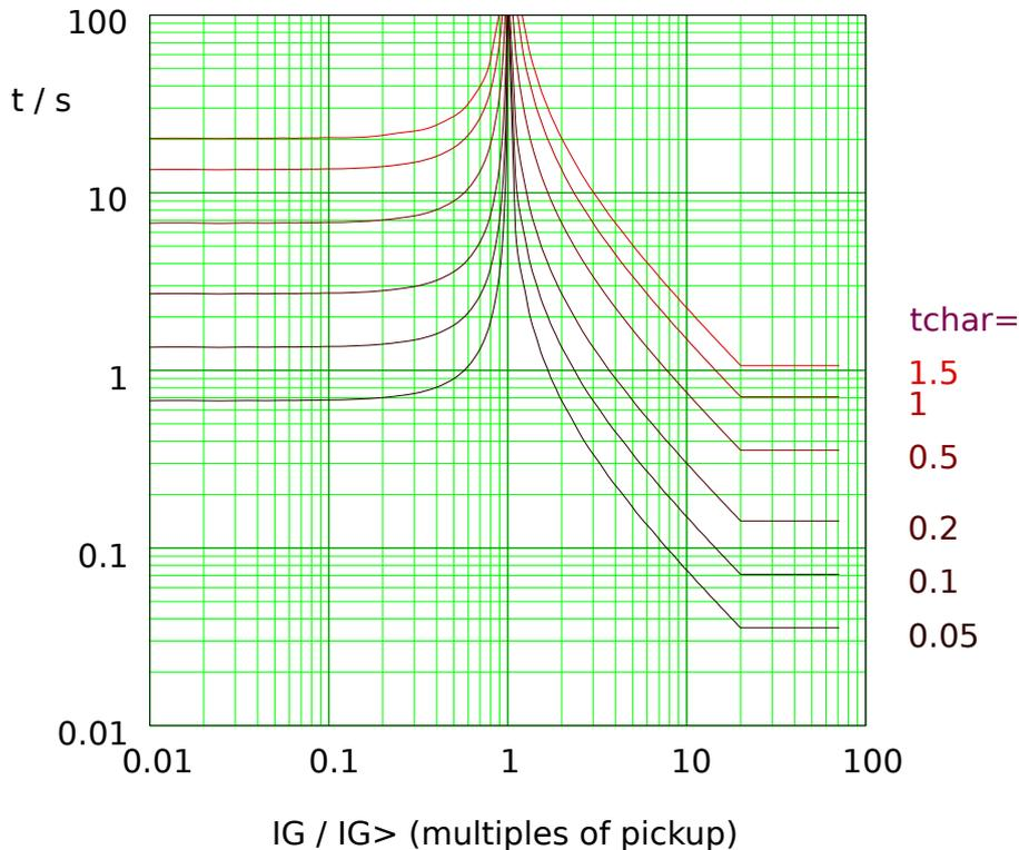
Fig. 58: VINV: reset delay (left half,  $I_G < I_{G>}$ ) and trip delay (right half,  $I_G > I_{G>}$ ), example for  $I_{G,max} = 20 \cdot I_{G>}$ .
