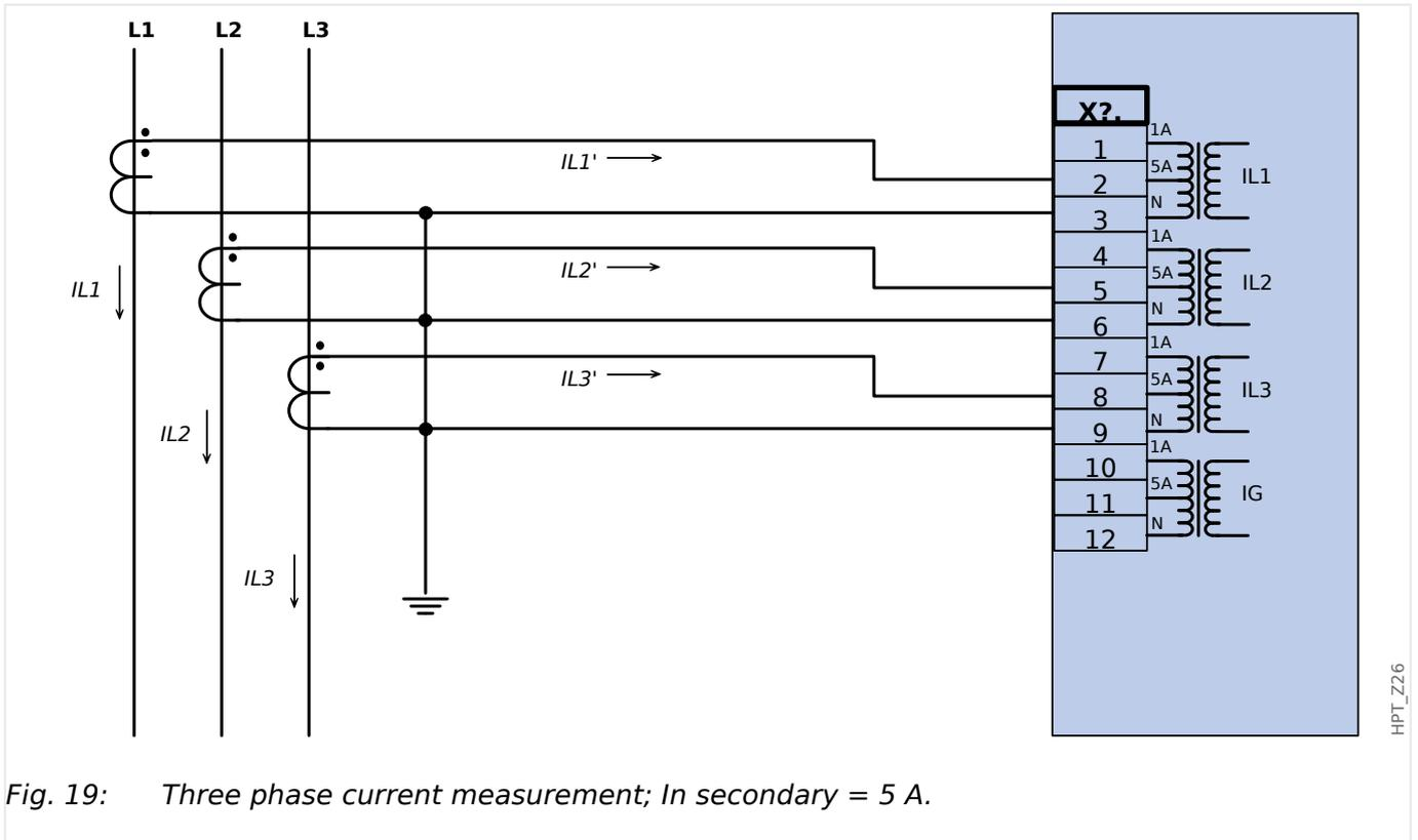
Fig. 19: Three phase current measurement; In secondary = 5 A.
