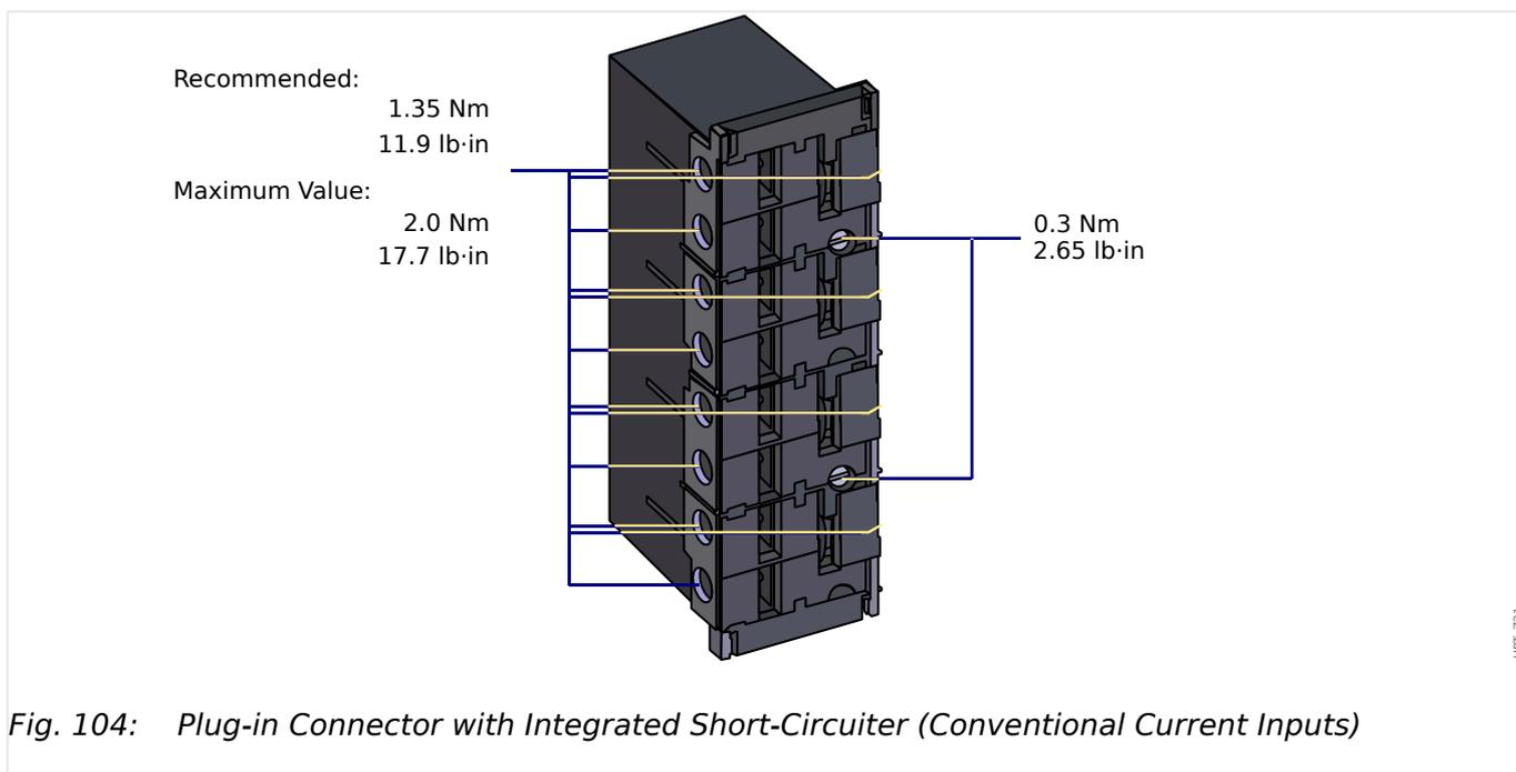
Fig. 104: Plug-in Connector with Integrated Short-Circuiter (Conventional Current Inputs)
