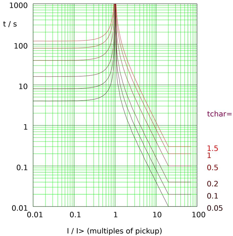
Fig. 47: EINV: reset delay (left half,  $I < I_N$ ) and trip delay (right half,  $I > I_N$ ), example for  $I_{max} = 20 \cdot I_N$ .
