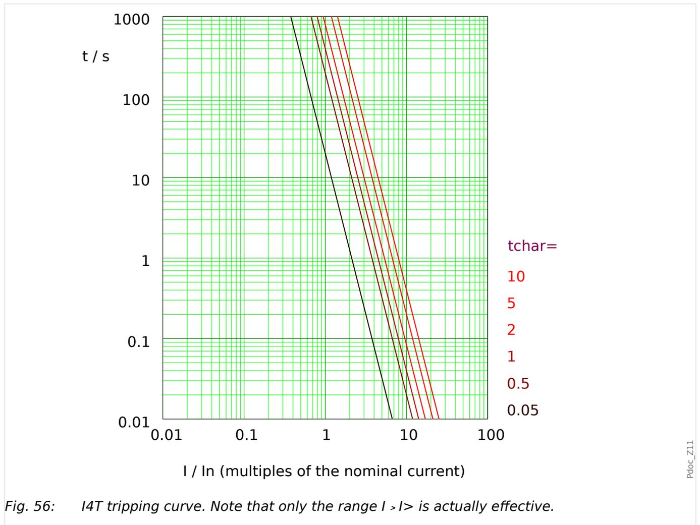
Fig. 56: I4T tripping curve. Note that only the range  $I > I_n$  is actually effective.
