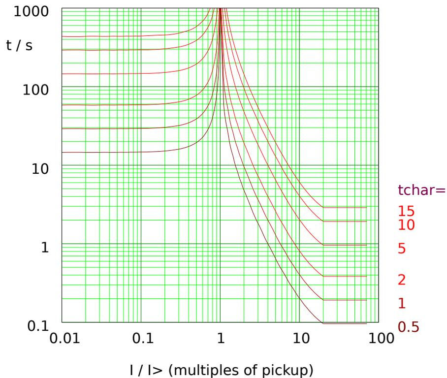
Fig. 51: EINV: reset delay (left half,  $I < I>$ ) and trip delay (right half,  $I > I>$ ), example for  $I_{max} = 20 \cdot I>$ .
