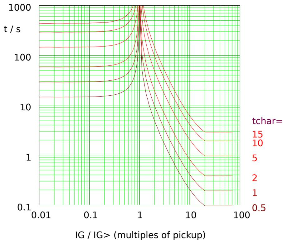
Fig. 90: EINV: reset delay (left half,  $I_G < I_{G>}$ ) and trip delay (right half,  $I_G > I_{G>}$ ), example for  $I_{G,max} = 20 \cdot I_{G>}$ .
