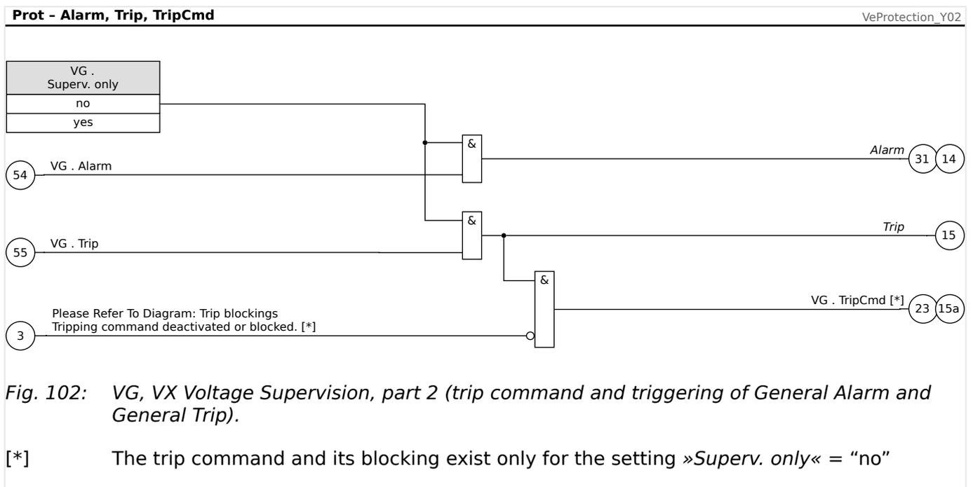
Fig. 102: VG, VX Voltage Supervision, part 2 (trip command and triggering of General Alarm and General Trip).
