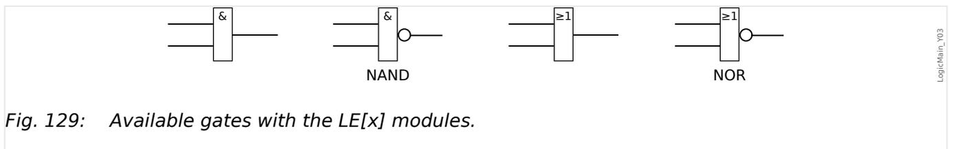
Fig. 129: Available gates with the LE[x] modules.
