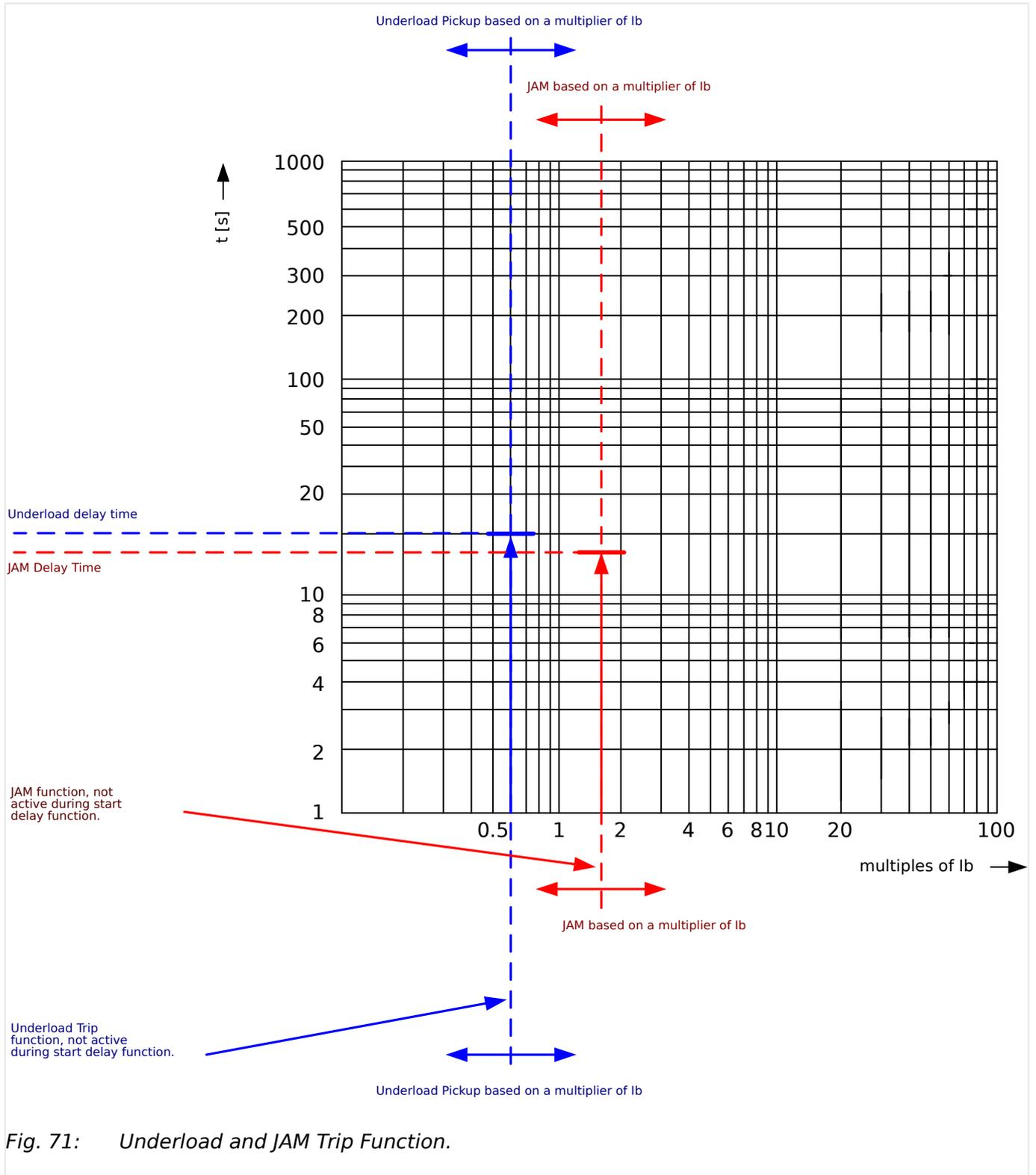
Fig. 71: Underload and JAM Trip Function.
