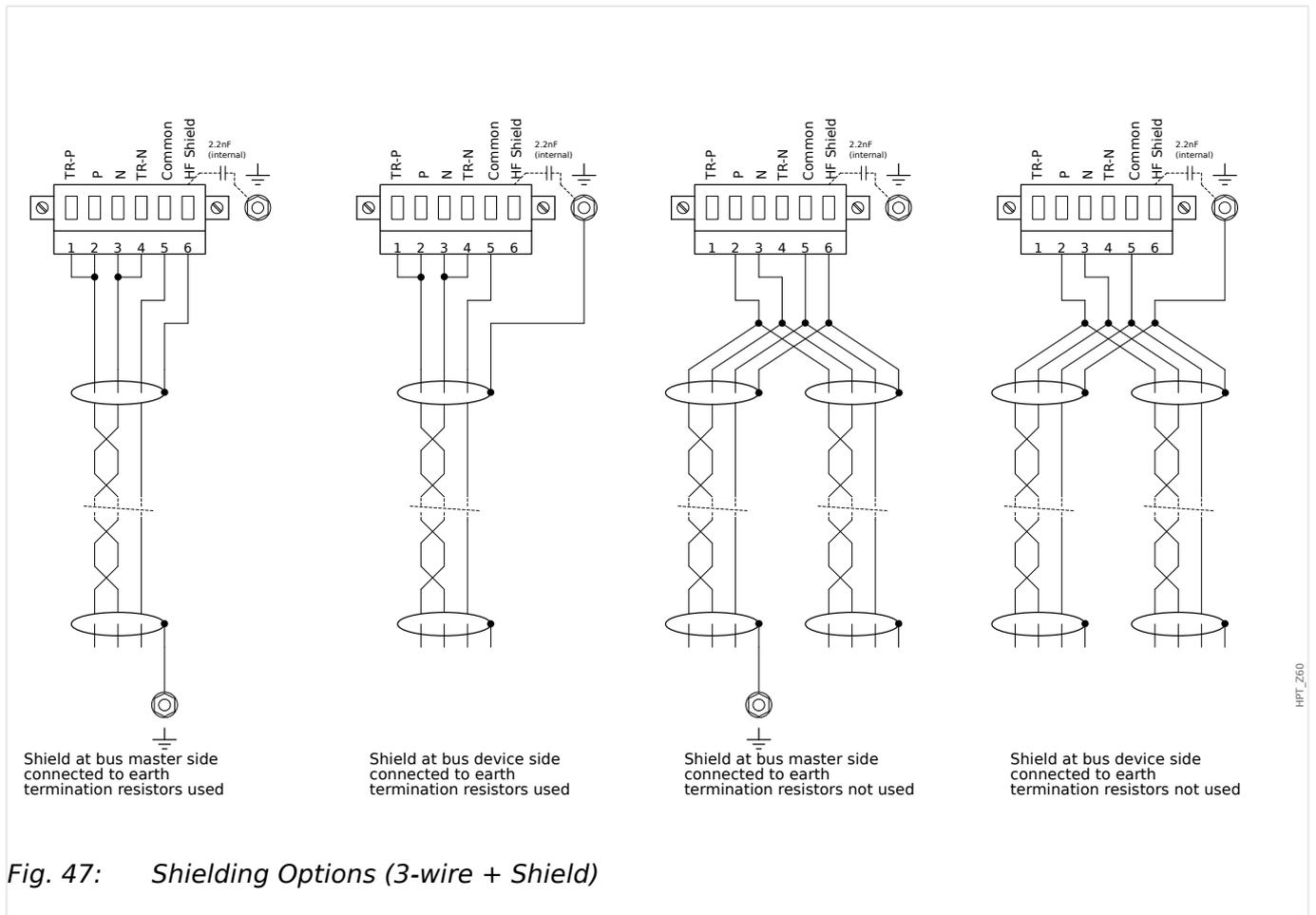
Fig. 47: Shielding Options (3-wire + Shield)
