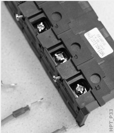
Move the slider aside, so that the screws and metal contact become fully accessible.
