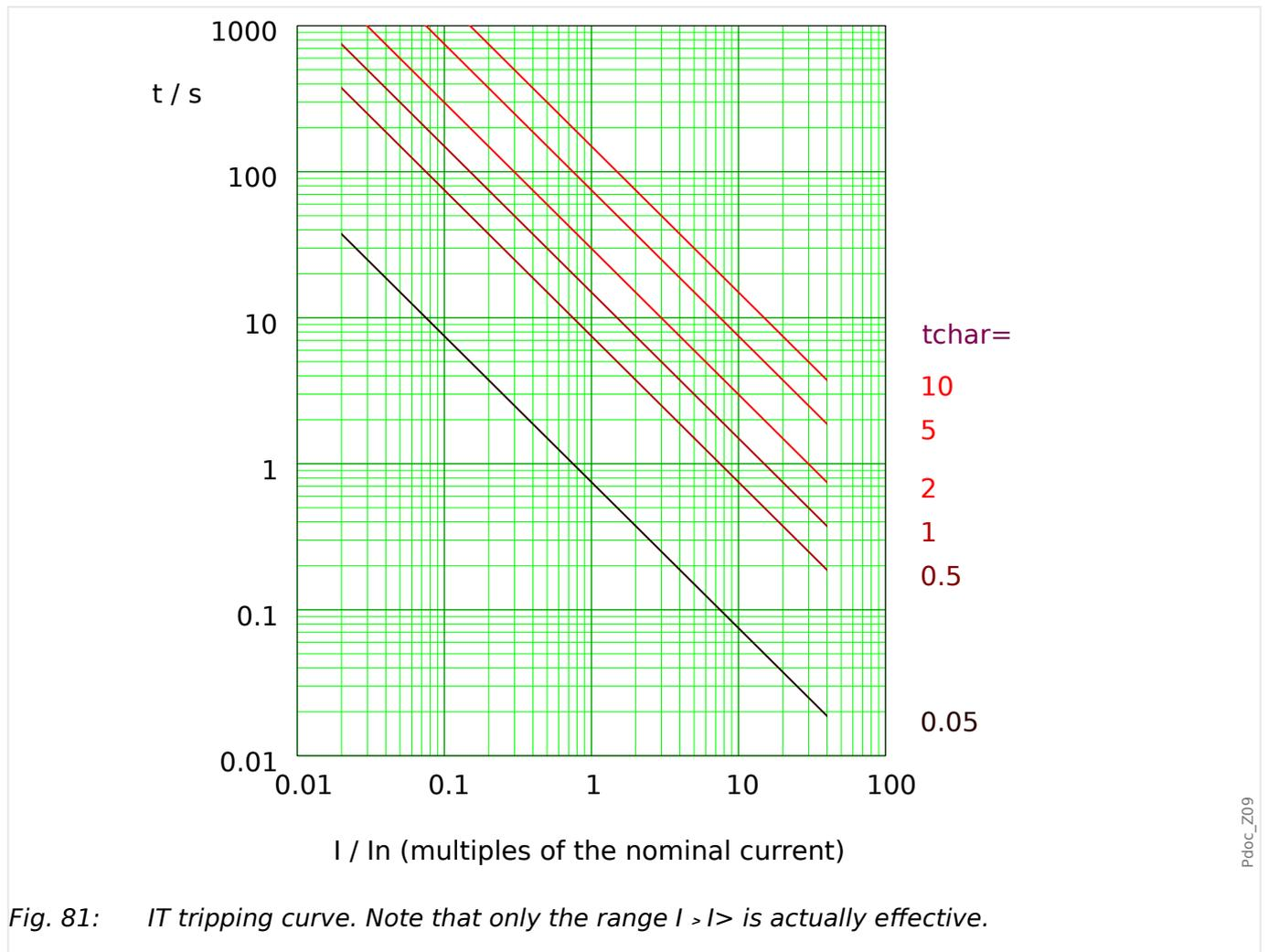
Fig. 81: IT tripping curve. Note that only the range  $I > I_n$  is actually effective.
