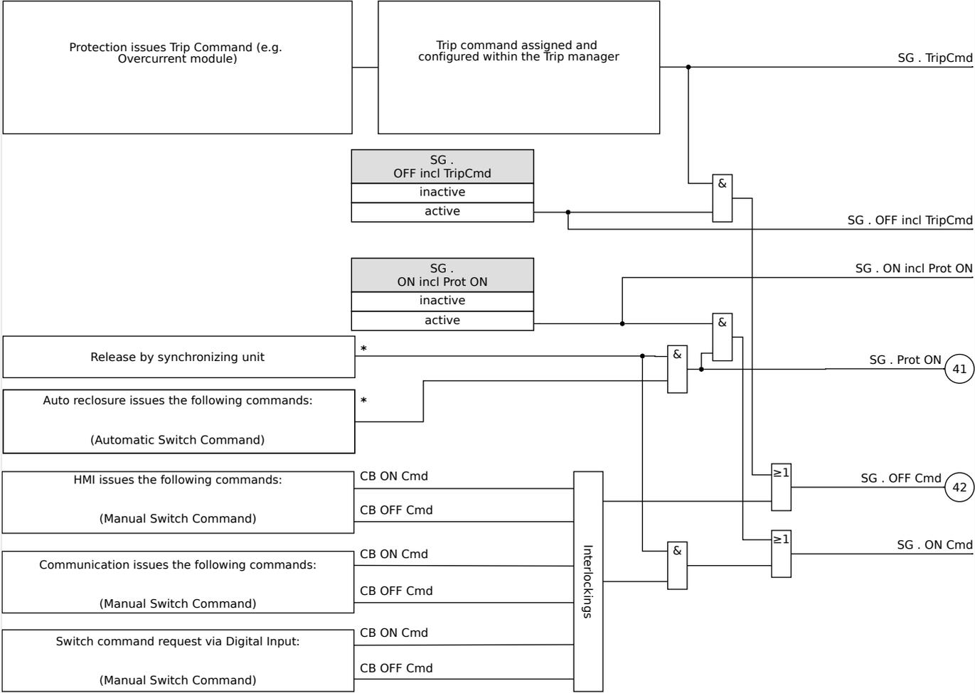
Fig. 119: Interlockings. (Parts labeled by “\*”: availability depends on ordered device type.)
