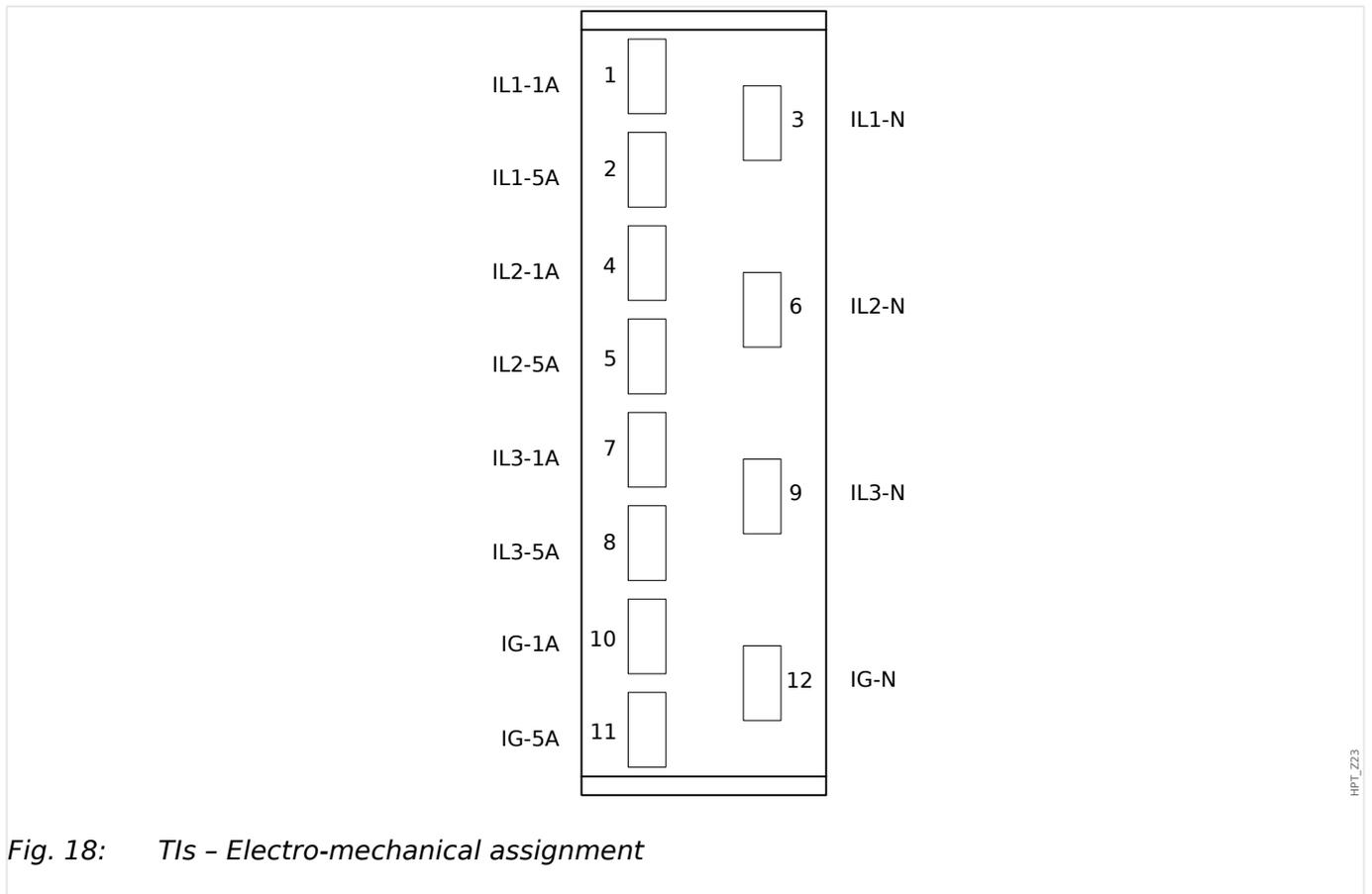
Fig. 18: TIs - Electro-mechanical assignment
