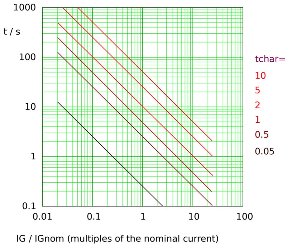
Fig. 94: IT tripping curve, example diagram for measured (non-sensitive) earth/ground current ( $5I_G$ ). Note that only the range  $I_G > I_G>$  is actually effective.
