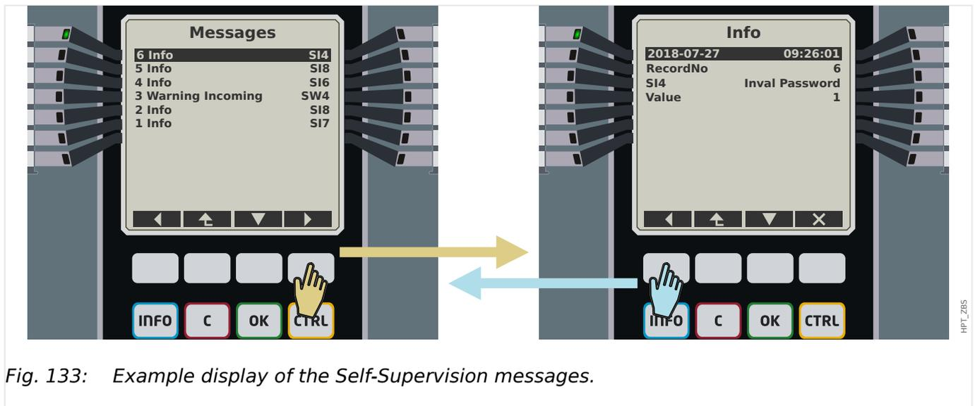
Fig. 133: Example display of the Self-Supervision messages.
