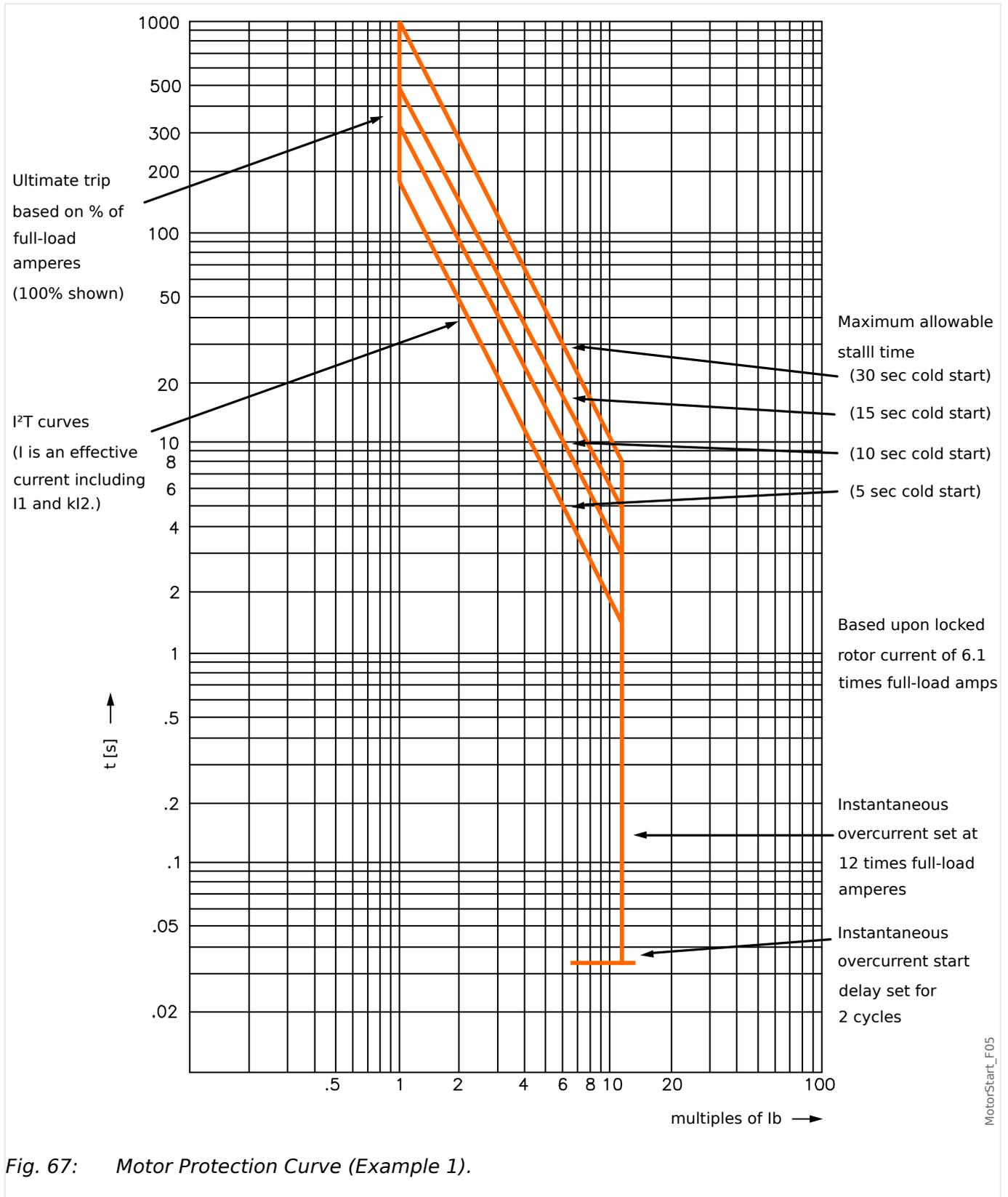
Fig. 67: Motor Protection Curve (Example 1).
