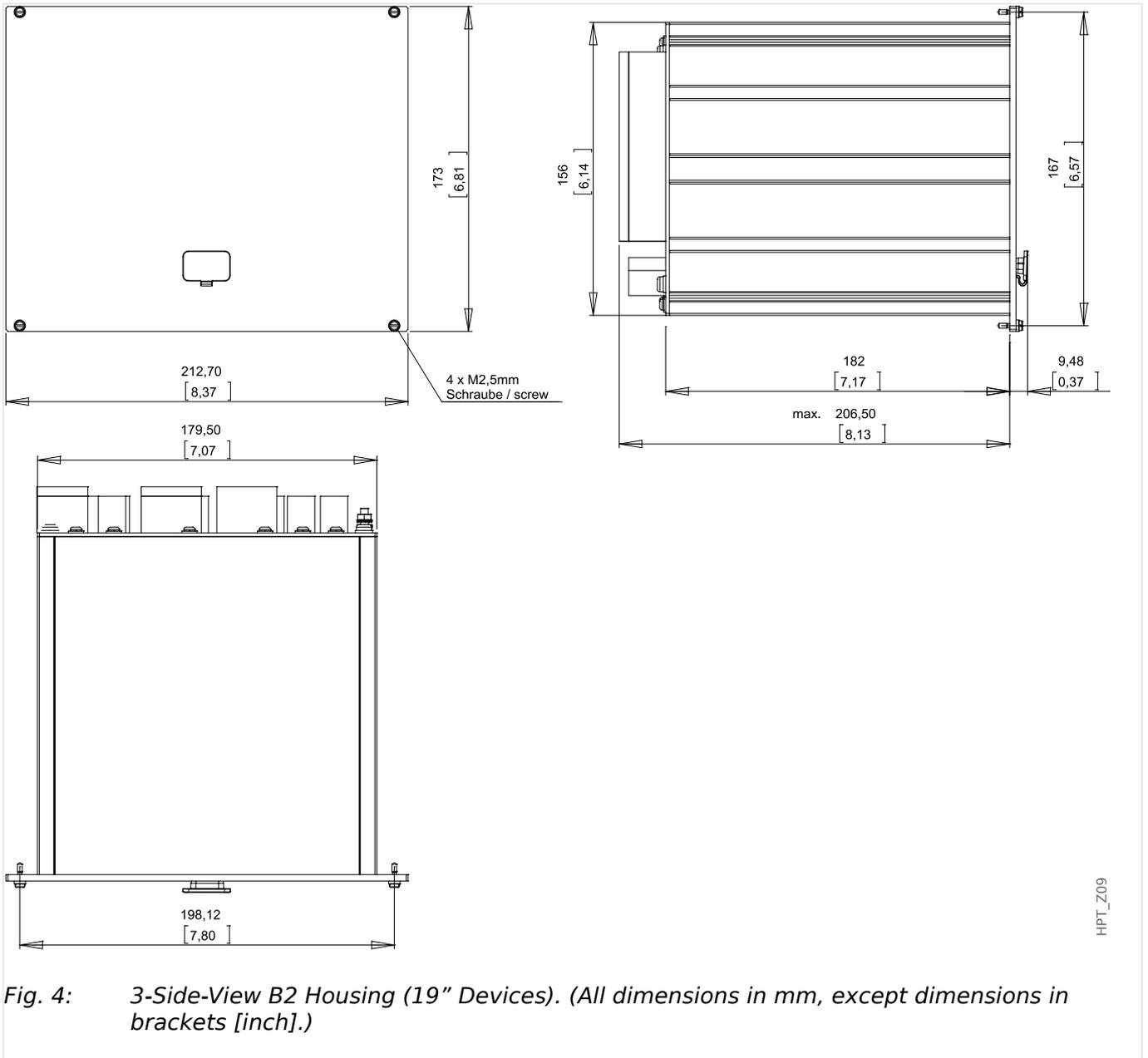
Fig. 4: 3-Side-View B2 Housing (19" Devices). (All dimensions in mm, except dimensions in brackets [inch].)
