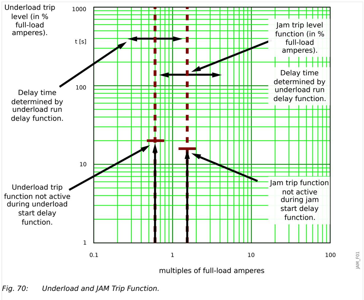
Fig. 70: Underload and JAM Trip Function.
