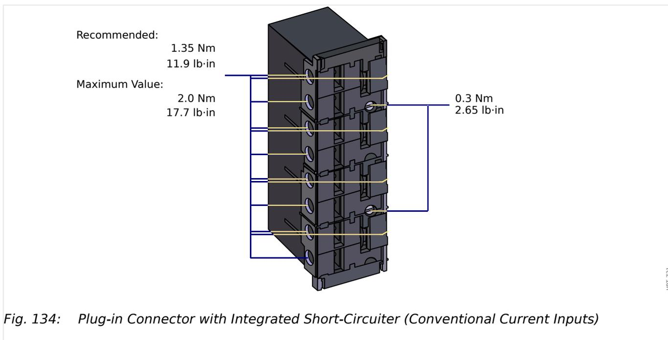
Fig. 134: Plug-in Connector with Integrated Short-Circuiter (Conventional Current Inputs)
