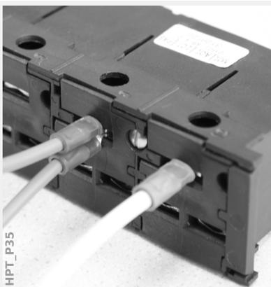
Remark: As long as the cable cross-sections are within the limits given in the Technical Data chapter ([↪ “12 Technical Data”, ↪ Table](#) ) it is also possible to insert two rings into one terminal, as shown here. This is useful for setting up the neutral point connection.
