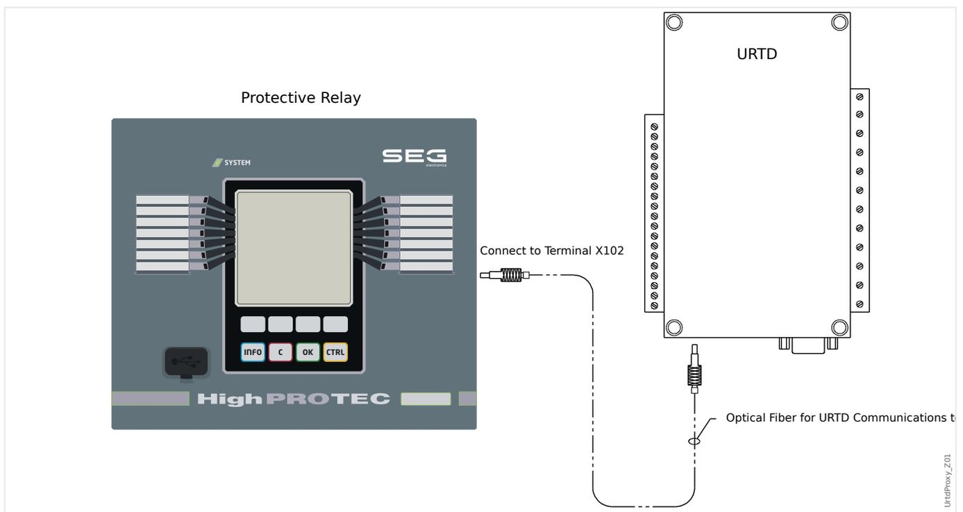
The figure above shows the fiber optic connections between the URTDII Module and the protective device. The protective device supports the optical fiber connection.
