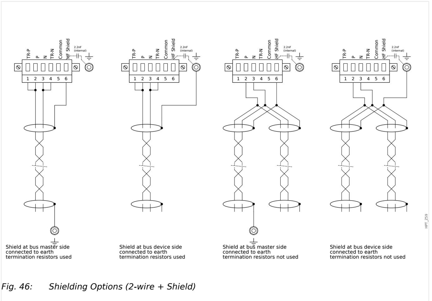
Fig. 46: Shielding Options (2-wire + Shield)
