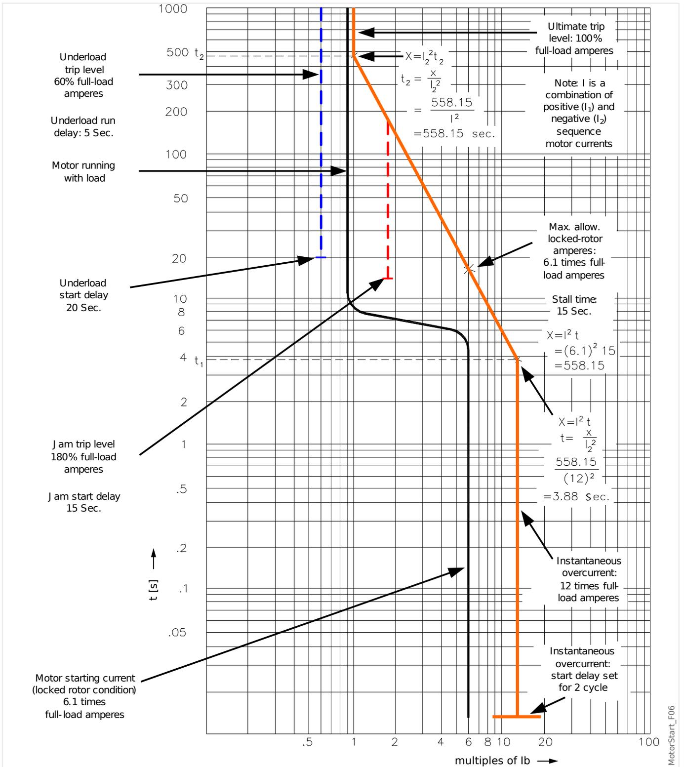
Fig. 68: Motor Protection Curve (Example 2 - without RTDs).
