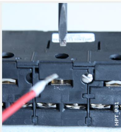
For the pin-terminal connection type, insert the cables and fasten them by the screws that are located at the side of the input card.
