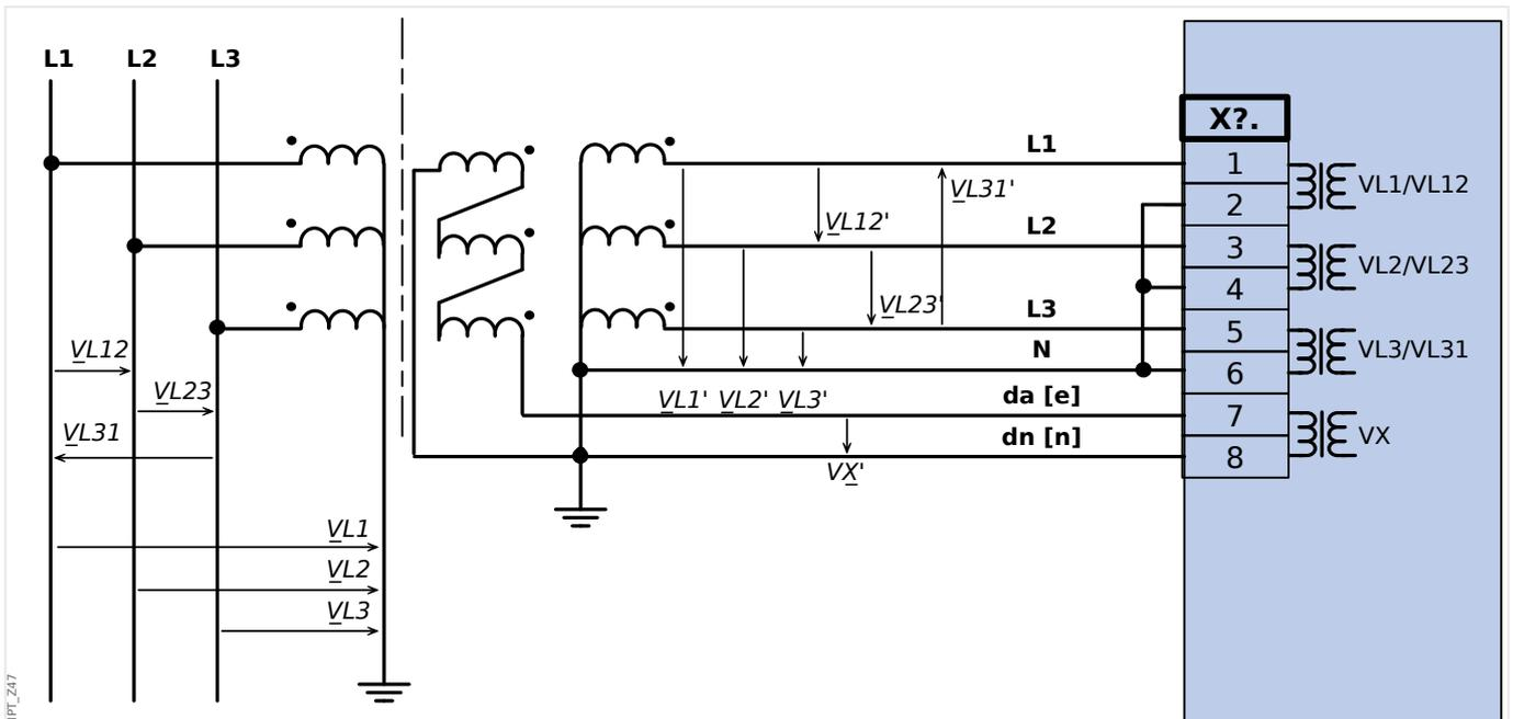
Fig. 29: VT Wye with Broken Delta Connection.
