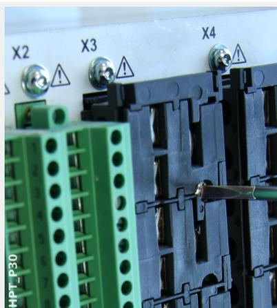
For either connection type, the first step is to remove the terminals from the device by opening the screws.
