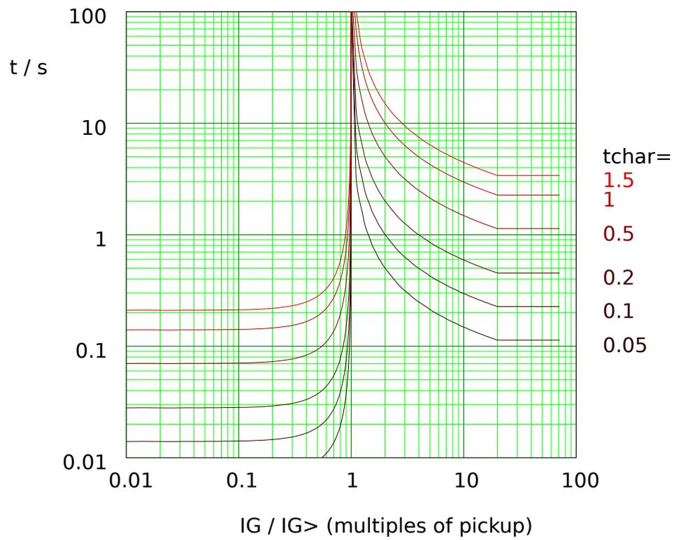
Fig. 84: NINV: reset delay (left half,  $I_G < I_{G>}$ ) and trip delay (right half,  $I_G > I_{G>}$ ), example for  $I_{G,max} = 20 \cdot I_{G>}$ .
