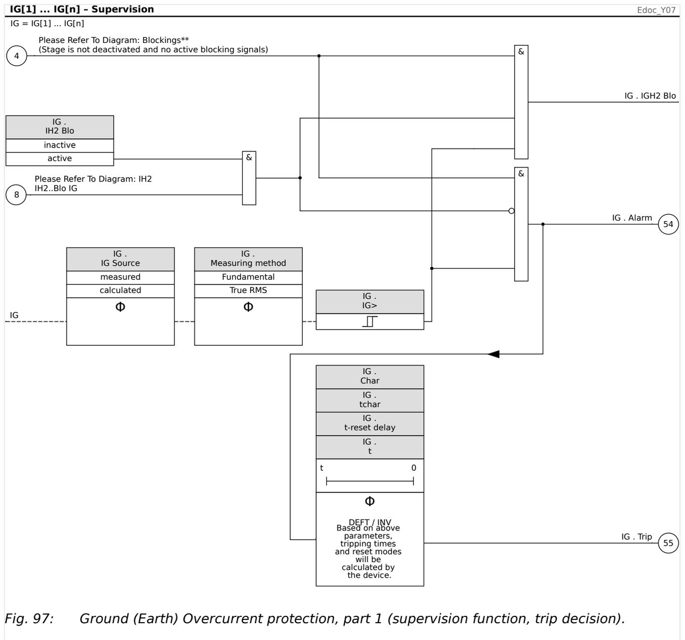
Fig. 97: Ground (Earth) Overcurrent protection, part 1 (supervision function, trip decision).
