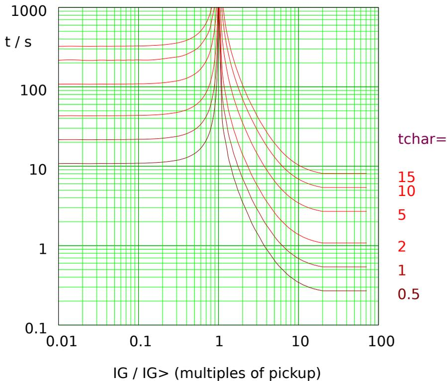
Fig. 89: VINV: reset delay (left half,  $I_G < I_{G>}$ ) and trip delay (right half,  $I_G > I_{G>}$ ), example for  $I_{G,max} = 20 \cdot I_{G>}$ .
