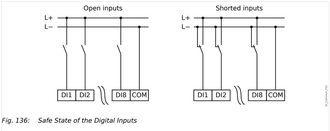
Fig. 136: Safe State of the Digital Inputs
