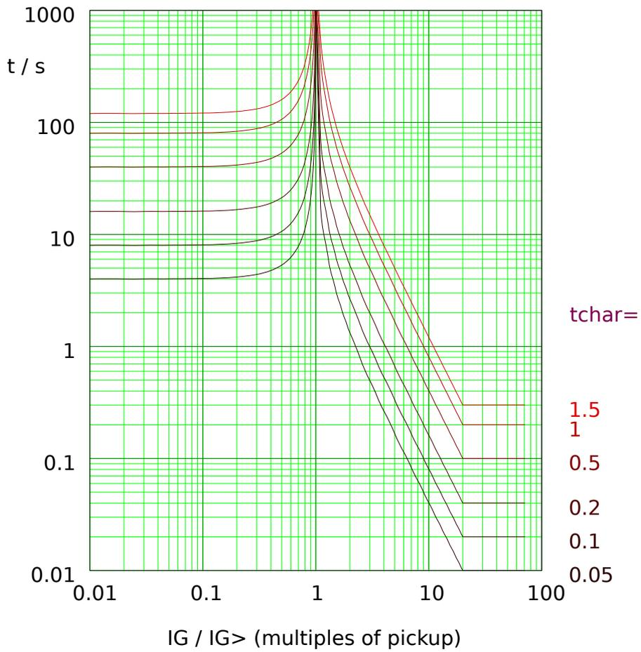
Fig. 86: EINV: reset delay (left half,  $I_G < I_{G>}$ ) and trip delay (right half,  $I_G > I_{G>}$ ), example for  $I_{G,max} = 20 \cdot I_{G>}$ .
