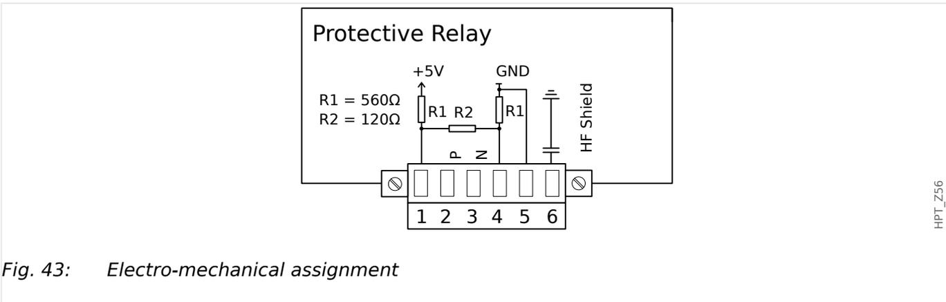
Fig. 43: Electro-mechanical assignment
