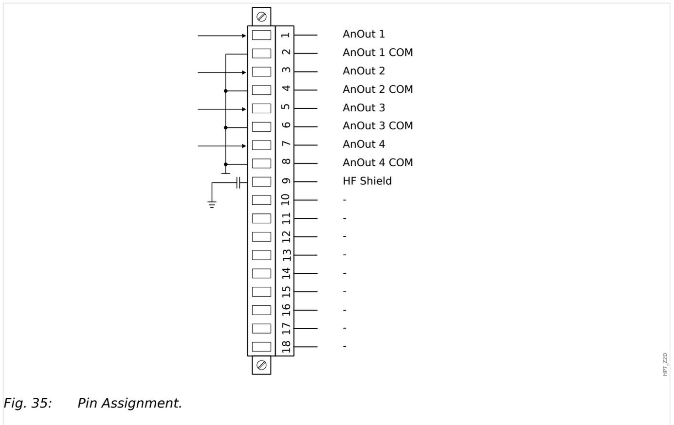
Fig. 35: Pin Assignment.
