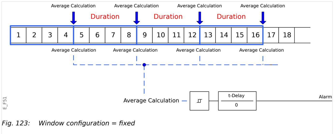
Fig. 123: Window configuration = fixed
