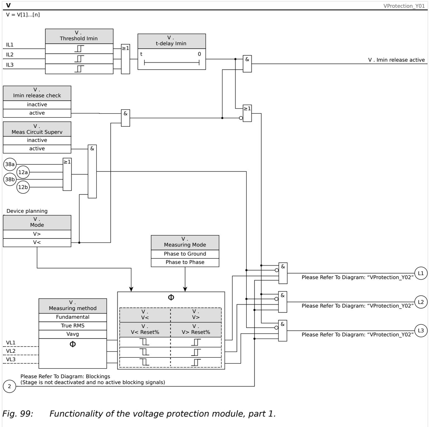
Fig. 99: Functionality of the voltage protection module, part 1.
