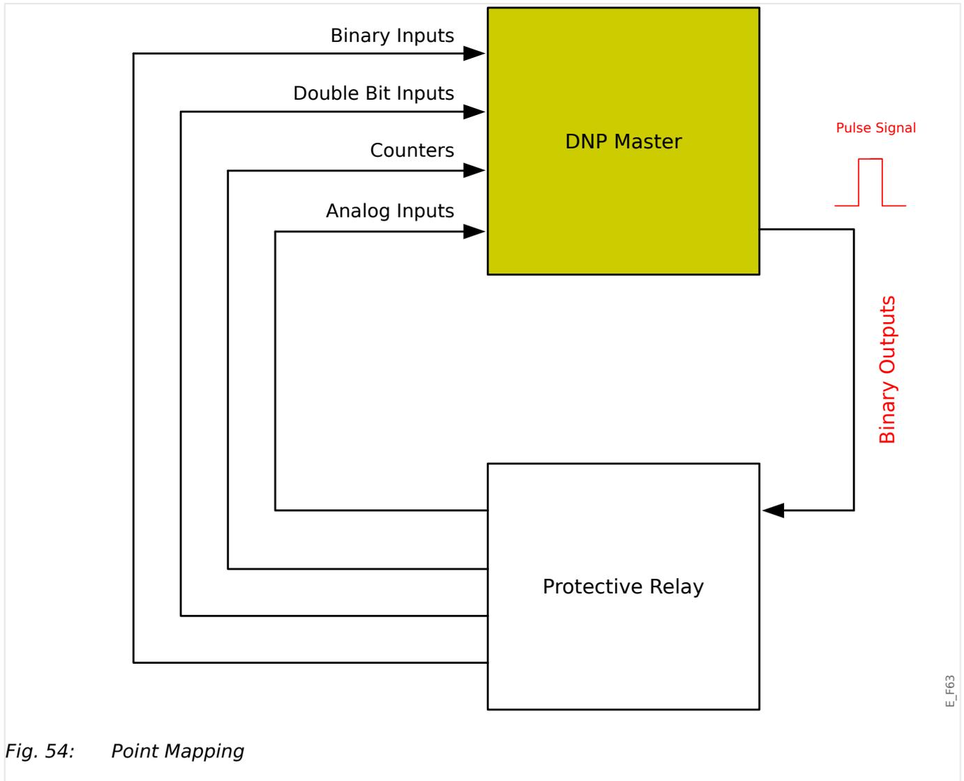
Fig. 54: Point Mapping
