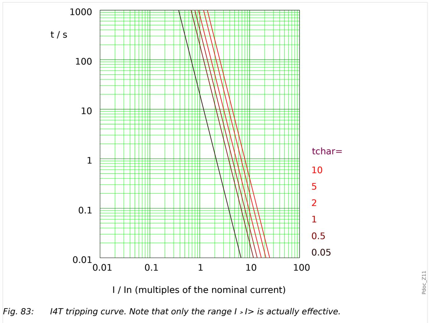
Fig. 83: I4T tripping curve. Note that only the range  $I > I_n$  is actually effective.
