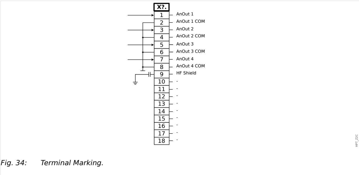
Fig. 34: Terminal Marking.
