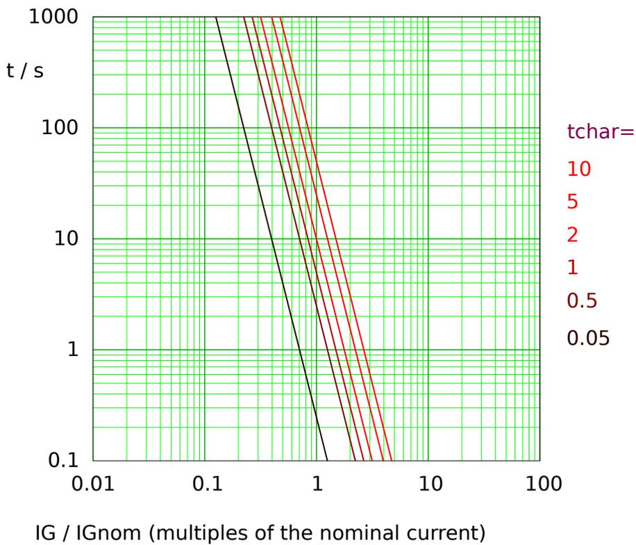
Fig. 96: I4T tripping curve, example diagram for measured (non-sensitive) earth/ground current (51G). Note that only the range  $I_G > I_G>$  is actually effective.
