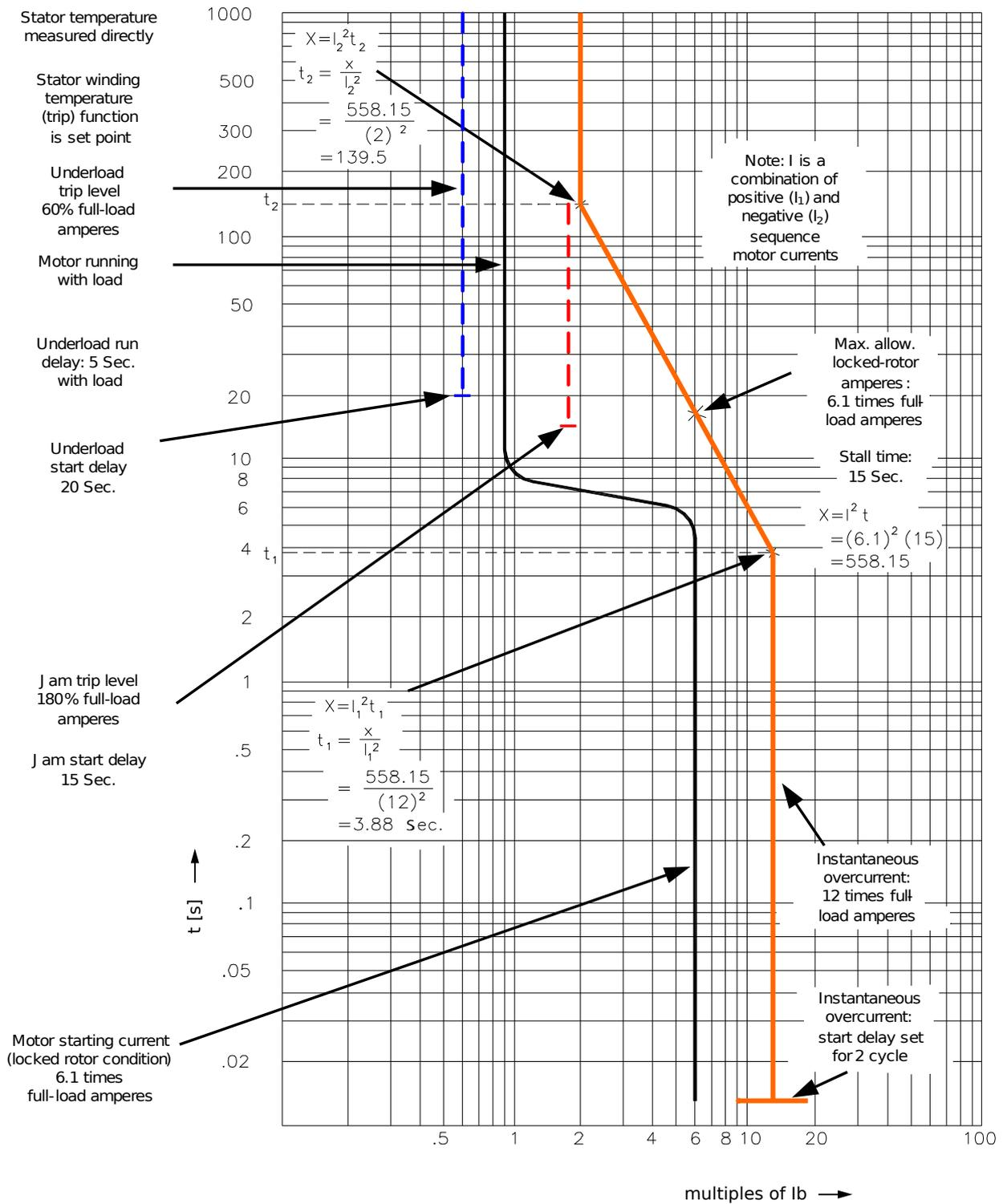
Fig. 69: Motor Protection Curve (Example 3 - with RTDs).
