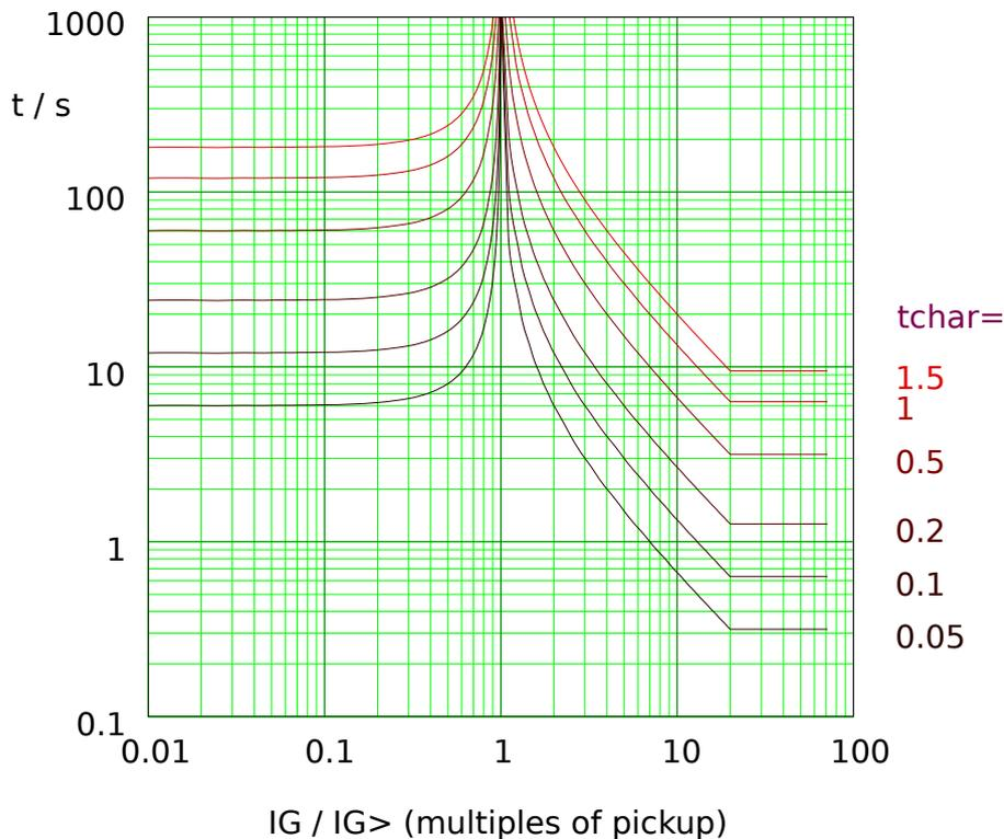
Fig. 87: LINV: reset delay (left half,  $I_G < I_{G>}$ ) and trip delay (right half,  $I_G > I_{G>}$ ), example for  $I_{G,max} = 20 \cdot I_{G>}$ .
