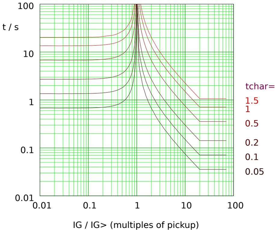
Fig. 85: VINV: reset delay (left half,  $I_G < I_{G>}$ ) and trip delay (right half,  $I_G > I_{G>}$ ), example for  $I_{G,max} = 20 \cdot I_{G>}$ .
