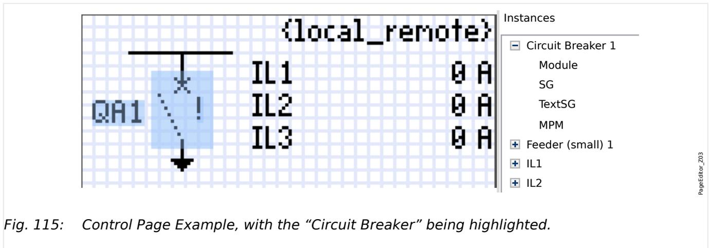
Fig. 115: Control Page Example, with the “Circuit Breaker” being highlighted.
