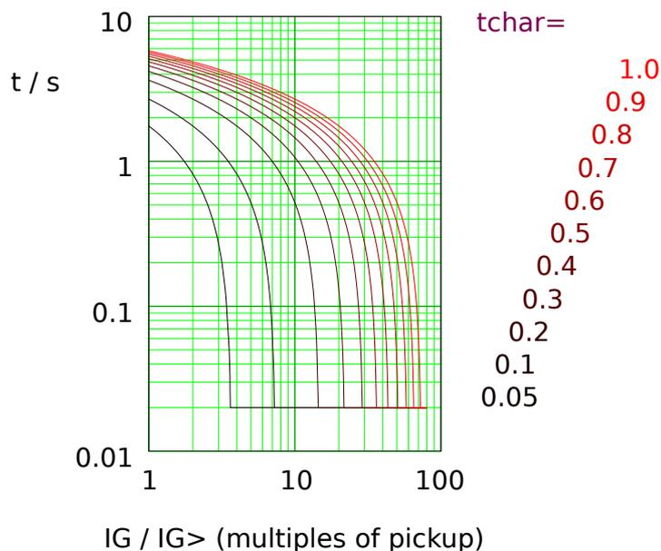
Fig. 92: RXIDG: trip delay,  $I_G > I_{G>}$ .
