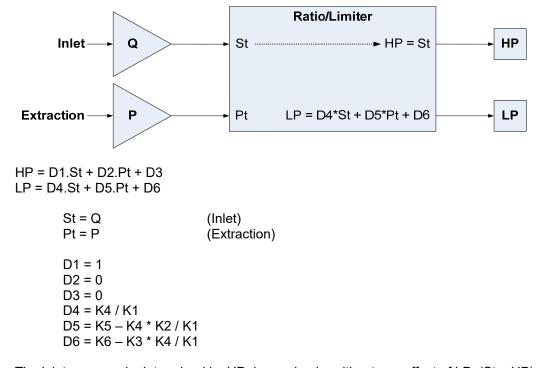
The inlet pressure is determined by HP demand only, without any effect of LP. (St = HP)
