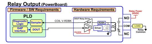
Figure 2-12. Relay Output Block Diagram
