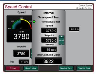
Figure 5-28. Internal (505) Overspeed Test
