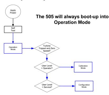
Figure 5-4. Control Mode Architecture
