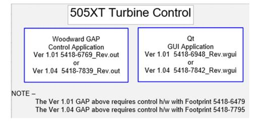
Figure 5-1. Software Architecture
