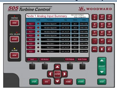
Figure 1-8. LinkNet Node 1 with 4 Vibration Signals
