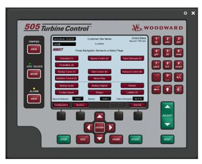
Figure 1-10. 505 Keypad and Display
