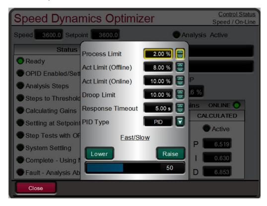
Figure 5-36. Configuration Parameters 'Configure' Pop-up
