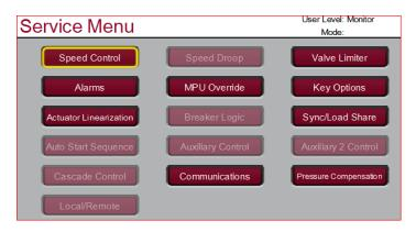
Figure 5-7. Service Menu Showing "Speed Control" IN-Focus
