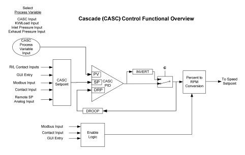
Figure 3-17. Cascade Functional Diagram
