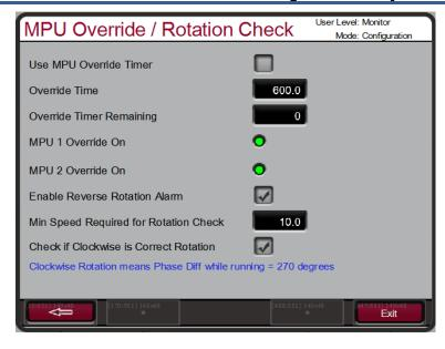
Figure 3-4. Speed Probe Rotation Check
