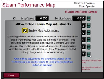
Figure 4-2a. Configuration Menu – On Line Steam Map Adjustments
