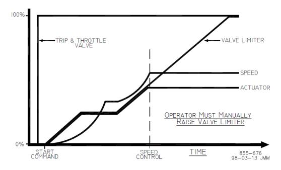
Figure 3-7. Semiautomatic Start Mode Example
