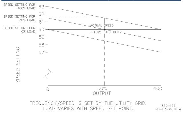
Figure 3-13. Frequency and Unit Load Relationship
