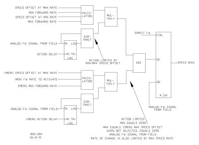
Figure 3-16. Typical Anti-surge Valve and Speed Feed-Forward Logic Trend
