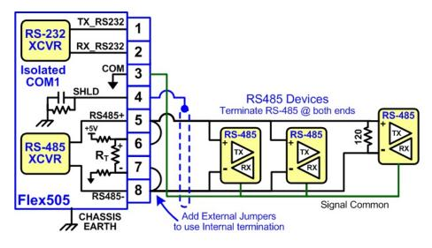
Figure 2-3. COM1 Example RS-485 Wiring
