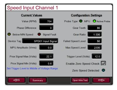
Figure 3-5. Speed Probe Zero Speed Detect
