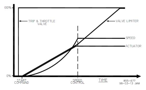
Figure 3-8. Automatic Start Mode Example
