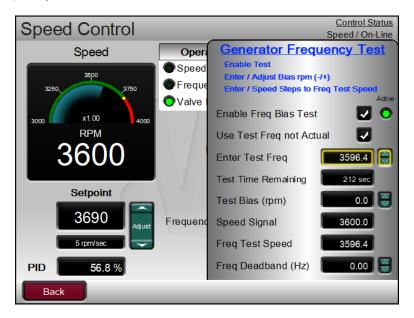
Figure 5-41. Generator Frequency Test PID Amount Increased
