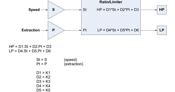
This mode is used when the two controlled parameters during normal operation are turbine speed/load and Extr/Adm pressure (or flow).
