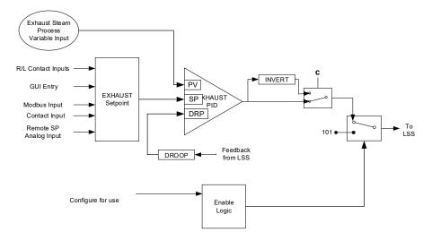
Figure 3-29. Exhaust Steam Pressure Control Overview
