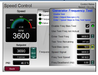
Figure 5-40. Generator Frequency Test PID Amount Decreased
