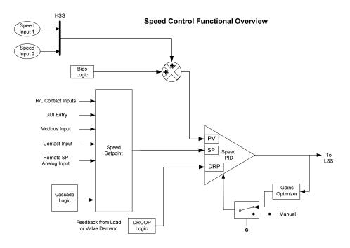
Figure 3-11. Speed Control Functional Diagram
