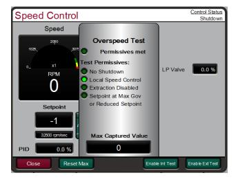
Figure 5-27. Overspeed Test Permissives
