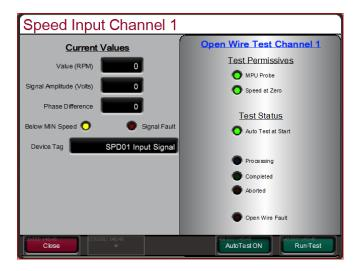
Figure 3-1. Open Wire Detection Test
