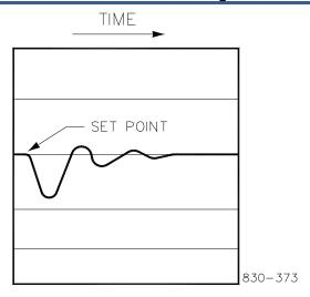
Figure 5-33. Typical Response to Load Change
