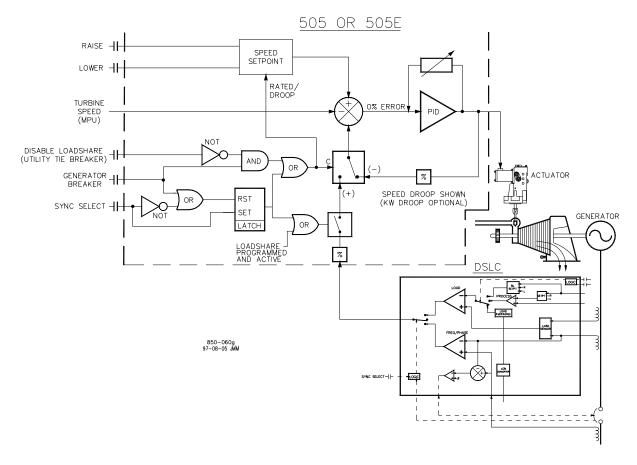
Figure 3-15. Load Sharing Logic
