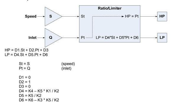
The inlet pressure is determined by HP demand only, without any effect of LP. (Pt = HP)
