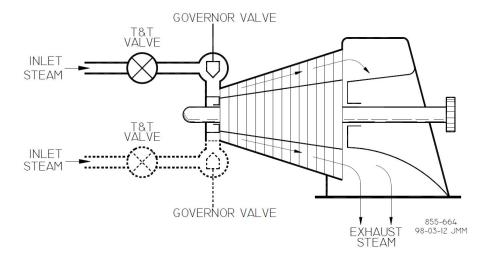
Figure 1-1. Typical Single or Dual Inlet Steam Turbine
