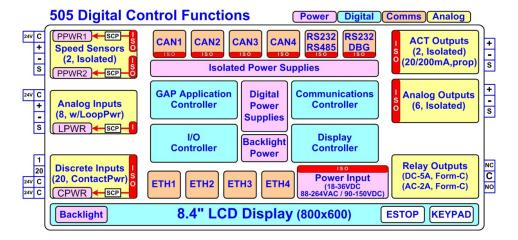
Figure 2-1. Functional Block Diagram (505 Control)
