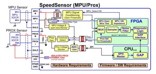
Figure 2-6. Speed Sensor Block Diagram
