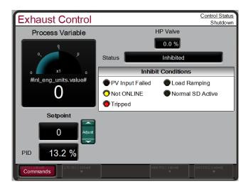
Figure 5-18. Exhaust Pressure Control Screen
