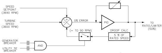
TURBINE INLET VALVE POSITION CONTROL WITH LOAD/FREQUENCY SWITCH
