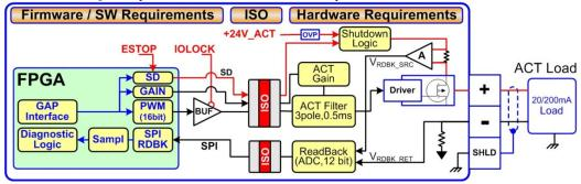
Figure 2-10. Actuator Output Block Diagram
