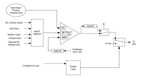
Figure 3-28. Inlet Steam Pressure Control Overview
