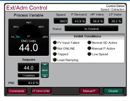
Figure 3-22. Extraction/Admission Control Panel
