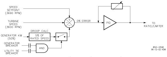
GENERATOR LOAD CONTROL (KW LOAD) WITH LOAD/FREQUENCY SWITCH
