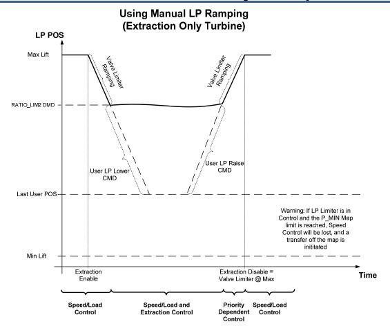
Figure 3-21. Transitions Between Speed Only and Ratio Limiter Control – Manual
