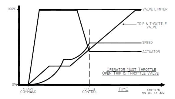
Figure 3-6. Manual Start Mode Example
