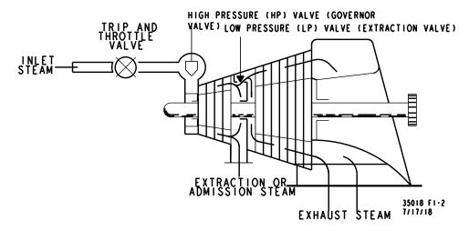
Figure 1-2. Typical Extraction and/or Admission Steam Turbine
