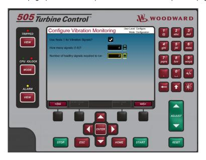
Figure 1-7. Vibration Wizard for LinkNet Node 1
