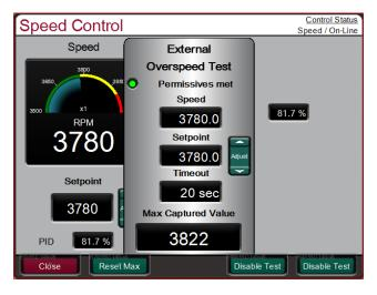
Figure 5-29. External Overspeed Test
