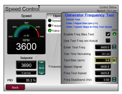
Figure 5-39. Generator Frequency Test "Active" LED Screen
