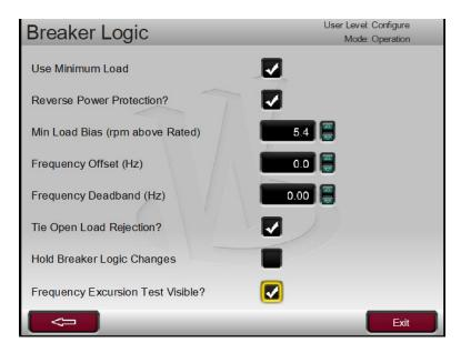
Figure 5-37. Breaker Logic Menu Screen
